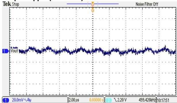
**Output Ripple (I<sub>Load</sub>=1A)**
