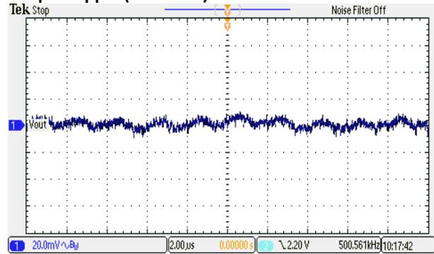
**Output Ripple (I<sub>Load</sub>=0A)**
