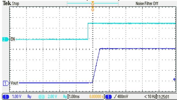
**Shut Down (I<sub>Load</sub>=1A)**
