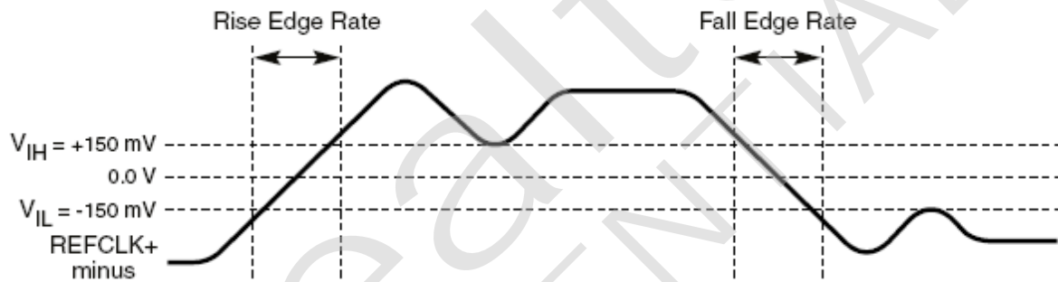
Figure 13. Differential Measurement Points for Rise and Fall Time
