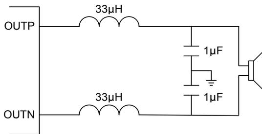
Figure 2. Typical LC Output Filter, Speaker Impedance=8Ω
