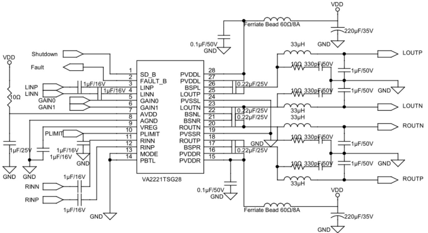
Figure 5. VA2221 Stereo Reference Application with LC Filter
