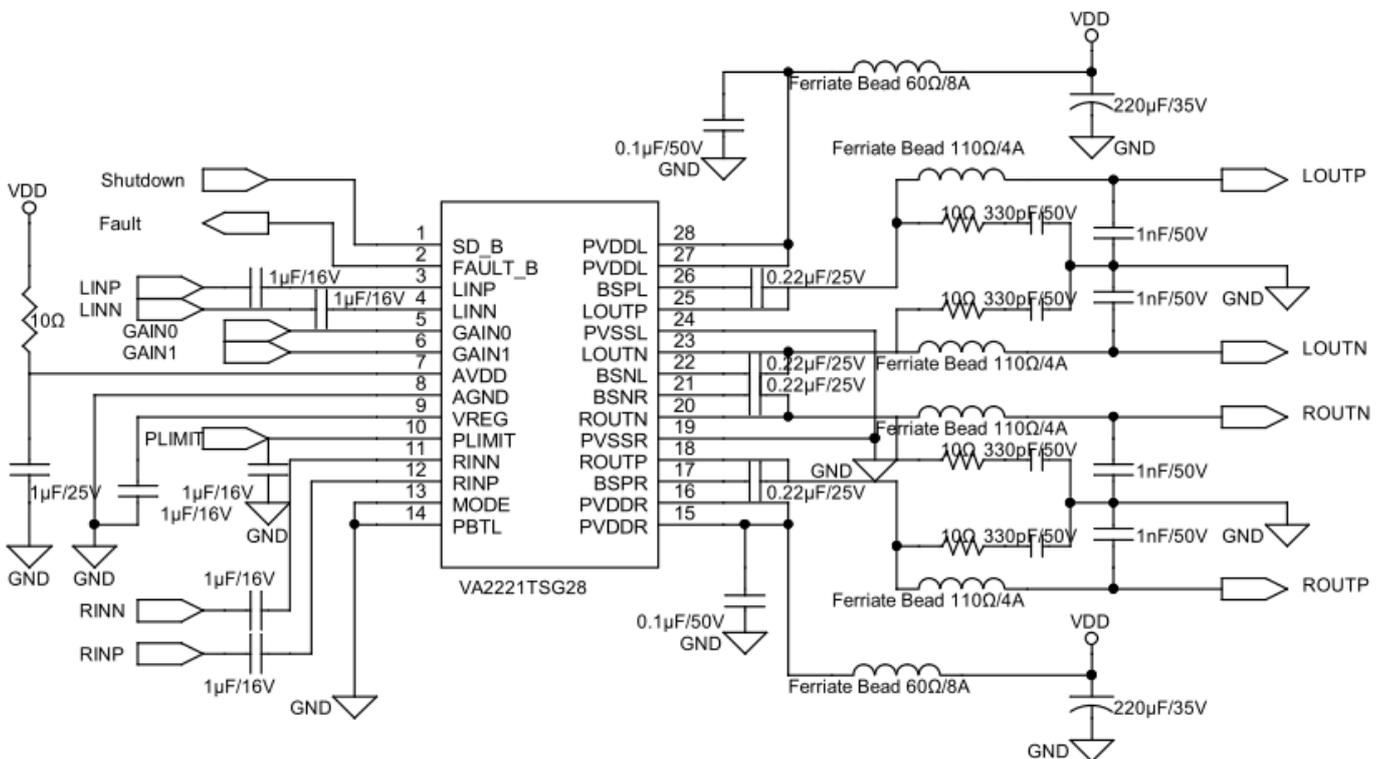
Figure 6. VA2221 Stereo Reference Application with Ferrite Bead
