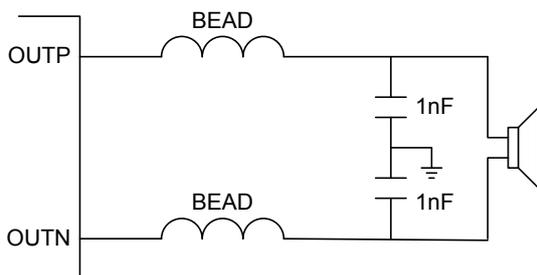
Figure 3. Typical Ferrite Chip Bead Output Filter
