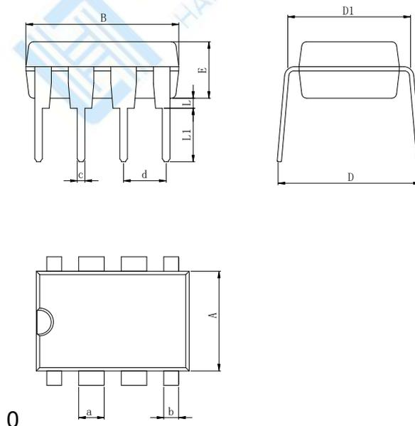
**Dimensions In Millimeters(DIP8L)**
