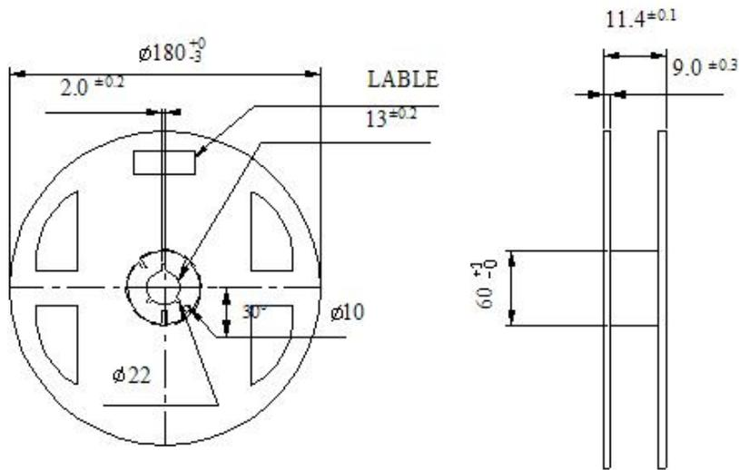
( Tolerance:  $\pm 0.2$ , Unit: mm )
