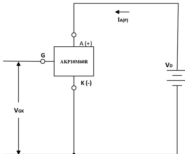
Fig.2. Current Regulator Controlled by V<sub>GK</sub>
