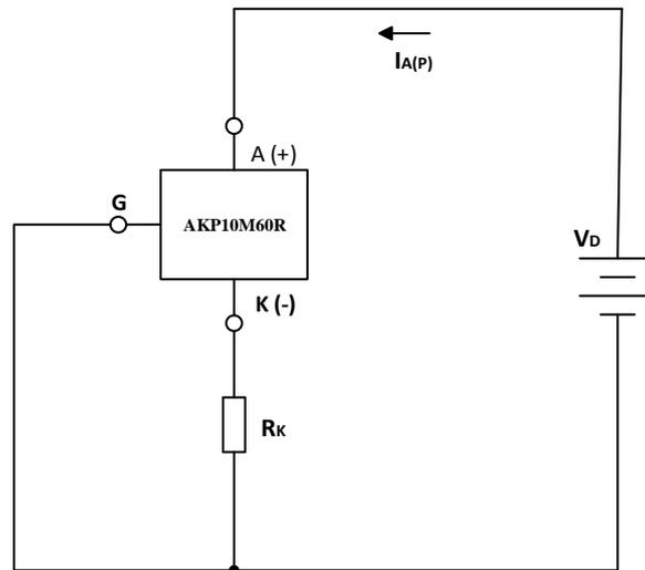
Fig.1. Resistor R<sub>k</sub> in Series with Negative Pin to Achieve Different Current Levels
