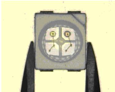
(3) When populating boards in SMT production, there are basically no restrictions regarding the form of the pick and place nozzle, except that mechanical pressure on the surface of the resin must be prevented. This is assured by choosing a pick and place nozzle which is larger than the LED's reflector area.
