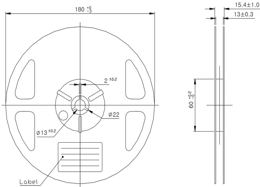
( Tolerance:  $\pm 0.2$ , Unit: mm )
