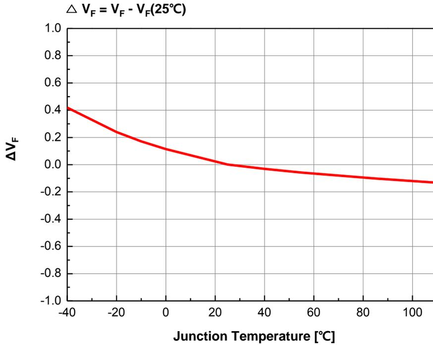
**Fig 7.2. Junction Temperature vs. Forward Voltage,  $I_F=20\text{mA}$  (Green)**
