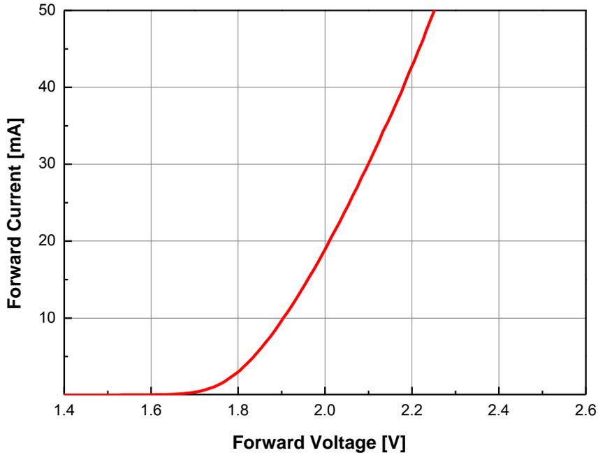
Fig 3.2. Forward Voltage vs. Forward Current,  $T_j=25^{\circ}\text{C}$  (Green)
