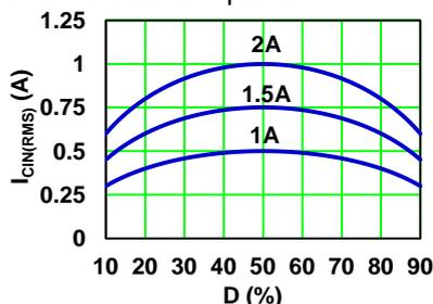
A low ESR capacitor is required to keep the noise minimum. Ceramic capacitors are better, but tantalum or low ESR electrolytic capacitors may also suffice. When using tantalum or electrolytic capacitors, a 0.1 $\mu$ F ceramic capacitor should be placed as close to the IC as possible.
