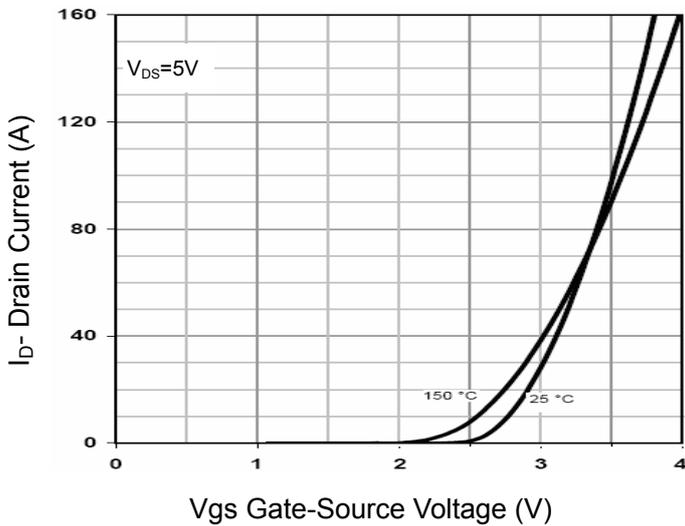
Figure 2 Transfer Characteristics
