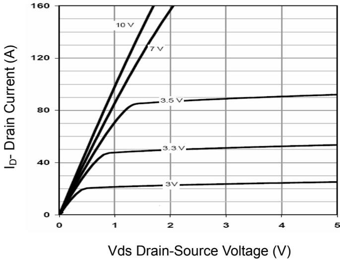
Figure 1 Output Characteristics
