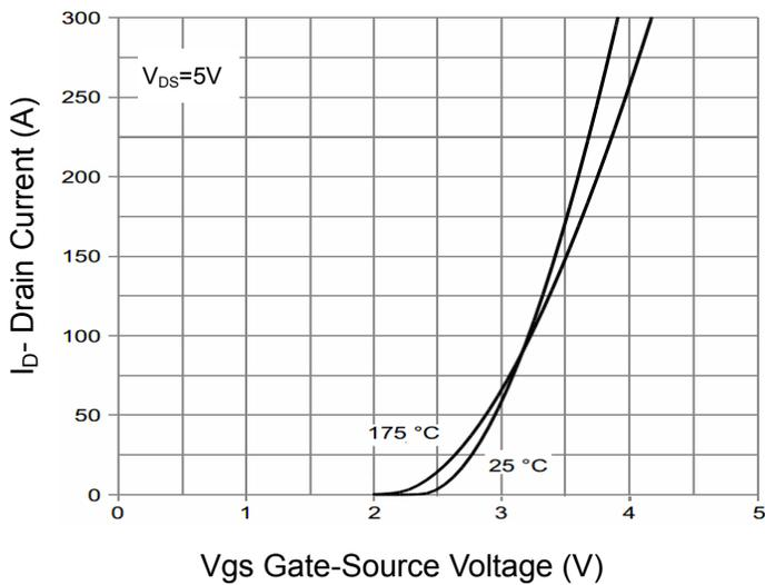
Figure 2 Transfer Characteristics
