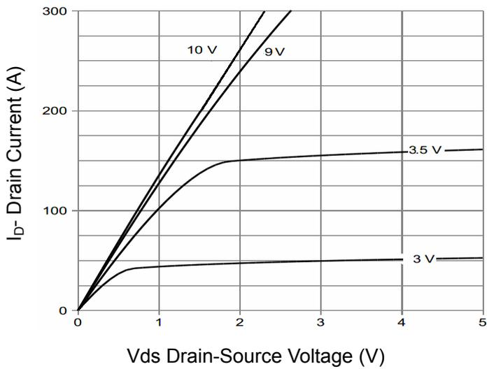
Figure 1 Output Characteristics
