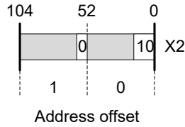
Figure 4-17. VCAP IP6PFX Entry Type-Group Fields
