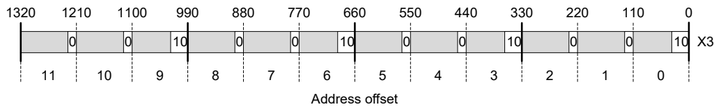
Figure 4-22. VCAP IS2 Action Type-Group Fields
