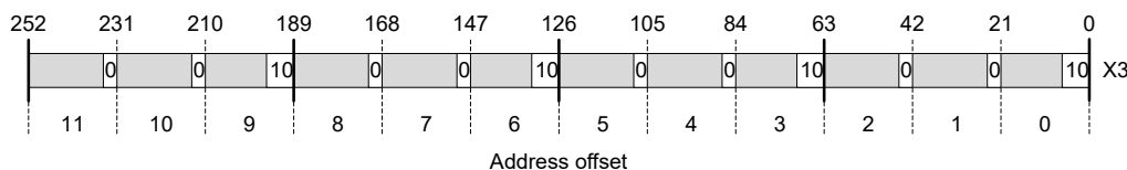
Figure 4-24. VCAP ES2 Action Type-Group Fields
