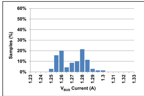
**FIGURE 2-16:** ILIM4 Trip Current Distribution<sup>(1)</sup>.
