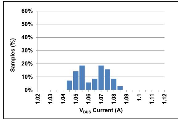
**FIGURE 2-15:** ILIM3 Trip Current Distribution<sup>(1)</sup>.
