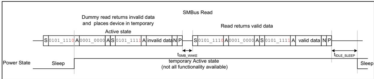
**FIGURE 5-2:** Wake from Sleep using SMBus Read.
