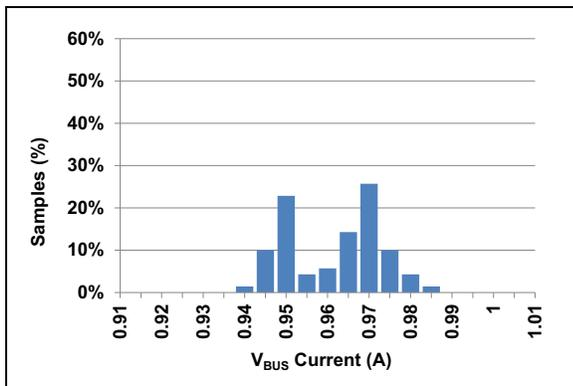
**FIGURE 2-14:** ILIM2 Trip Current Distribution<sup>(1)</sup>.
