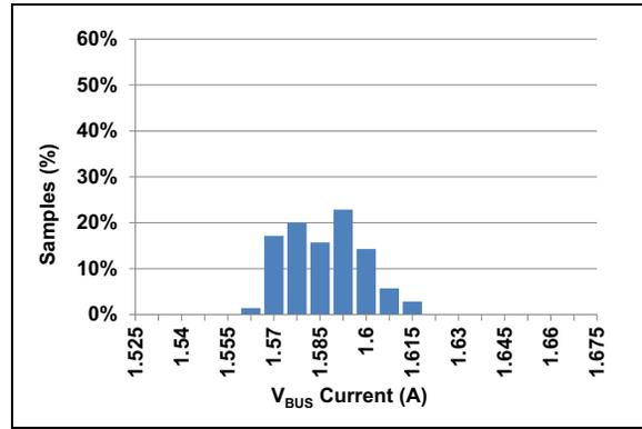
**FIGURE 2-17:** ILIM5 Trip Current Distribution<sup>(1)</sup>.
