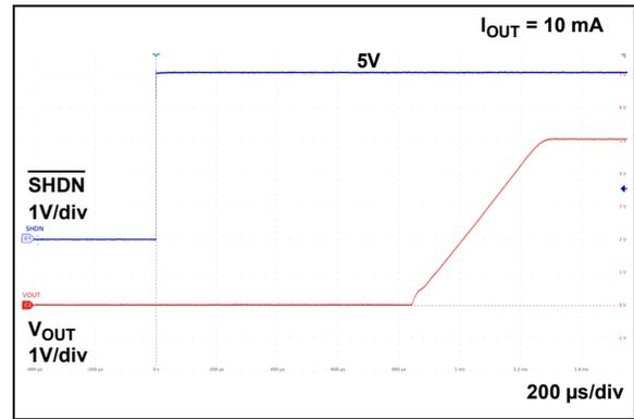
**FIGURE 2-33:** Start-up From  $\overline{\text{SHDN}}$  ( $V_R = 5.0\text{V}$ ).
