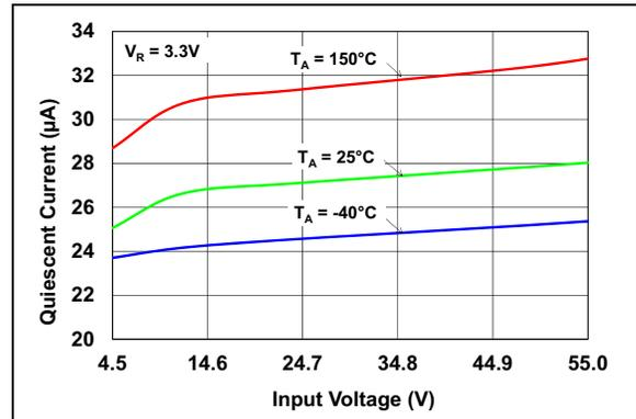
**FIGURE 2-10:** Quiescent Current vs. Input Voltage ( $V_R = 3.3\text{V}$ ).
