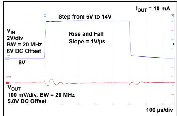
**FIGURE 2-27:** Dynamic Line Step ( $V_R = 5.0\text{V}$ ).
