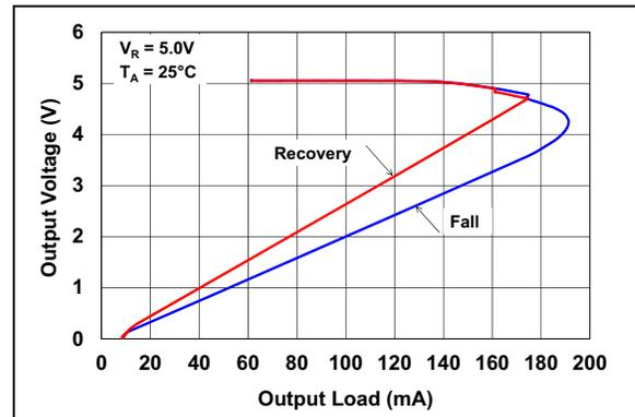
**FIGURE 2-17:** Current Foldback ( $V_R = 5.0\text{V}$ ).
