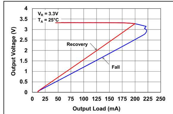
**FIGURE 2-16:** Current Foldback ( $V_R = 3.3\text{V}$ ).
