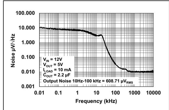
**FIGURE 2-21:** Noise vs. Frequency ( $V_R = 5.0\text{V}$ ).
