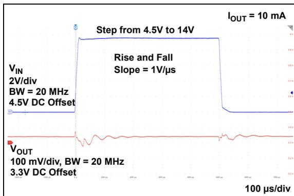
**FIGURE 2-26:** Dynamic Line Step ( $V_R = 3.3\text{V}$ ).
