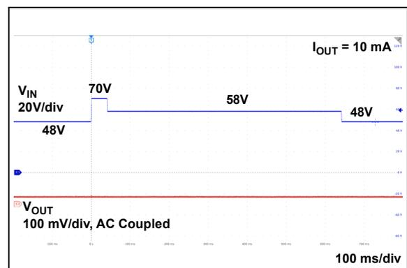
**FIGURE 2-34:** Overvoltage Line Transient Response ( $V_R = 5\text{V}$ ).
