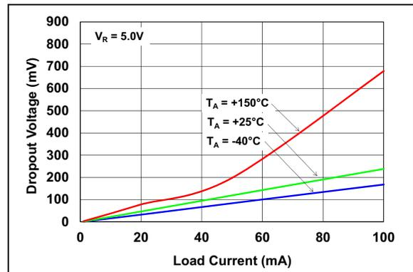
**FIGURE 2-5:** Dropout Voltage vs. Load Current ( $V_R = 5.0\text{V}$ ).
