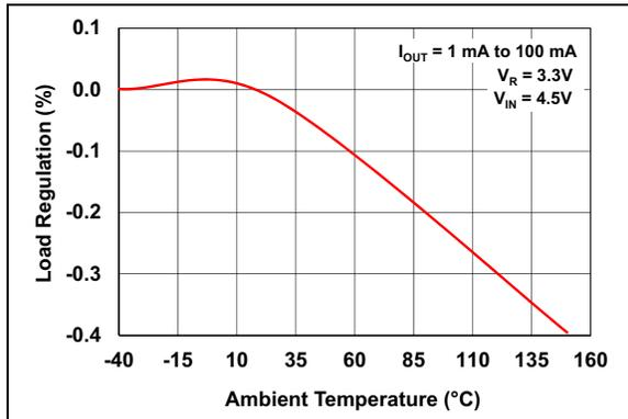
**FIGURE 2-7:** Load Regulation vs. Temperature ( $V_R = 3.3\text{V}$ ).
