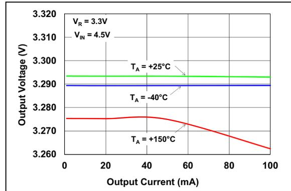
**FIGURE 2-4:** Output Voltage vs. Output Current ( $V_R = 3.3\text{V}$ ).
