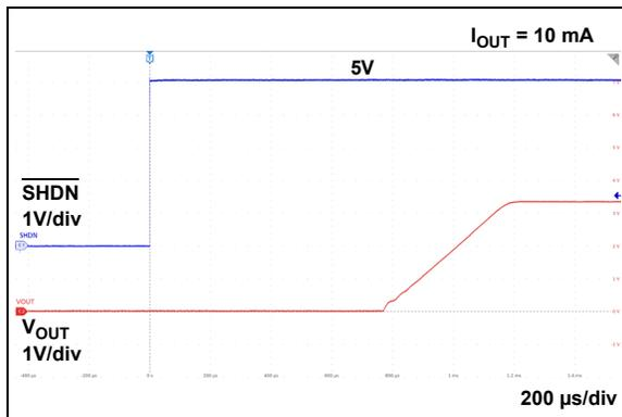
**FIGURE 2-32:** Start-up From  $\overline{\text{SHDN}}$  ( $V_R = 3.3\text{V}$ ).
