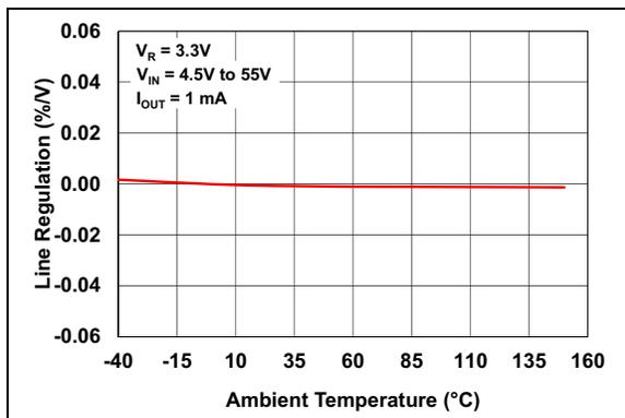
**FIGURE 2-9:** Line Regulation vs. Ambient Temperature ( $V_R = 3.3\text{V}$ ).
