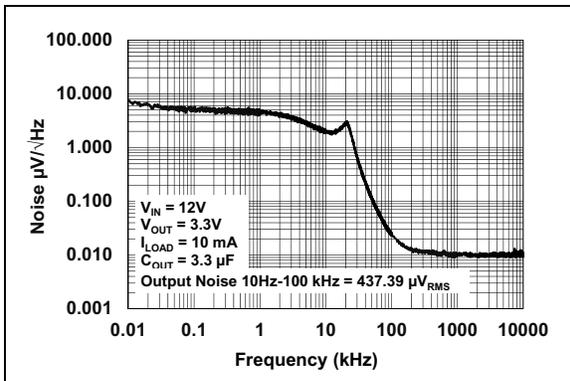
**FIGURE 2-20:** Noise vs. Frequency ( $V_R = 3.3\text{V}$ ).
