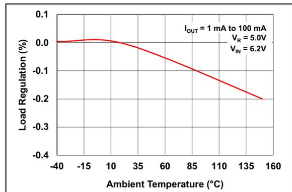
**FIGURE 2-6:** Load Regulation vs. Temperature ( $V_R = 5.0\text{V}$ ).
