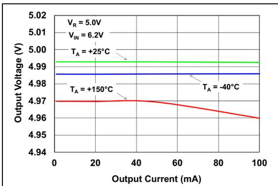
**FIGURE 2-3:** Output Voltage vs. Output Current ( $V_R = 5.0\text{V}$ ).
