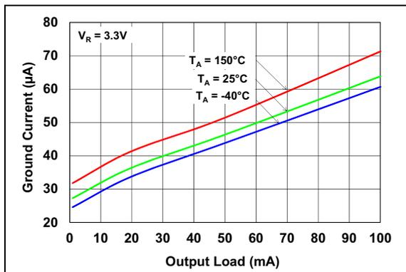
**FIGURE 2-14:** Ground Current vs. Output Current ( $V_R = 3.3\text{V}$ ).
