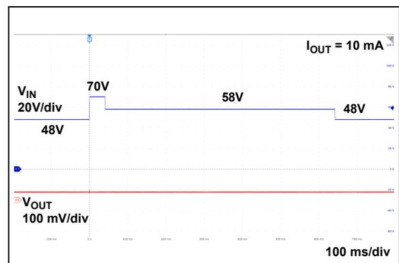
**FIGURE 2-35:** Overvoltage Line Transient Response ( $V_R = 3.3\text{V}$ ).
