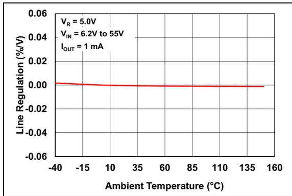
**FIGURE 2-8:** Line Regulation vs. Ambient Temperature ( $V_R = 5.0\text{V}$ ).
