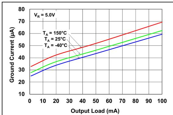
**FIGURE 2-15:** Ground Current vs. Output Current ( $V_R = 5.0\text{V}$ ).
