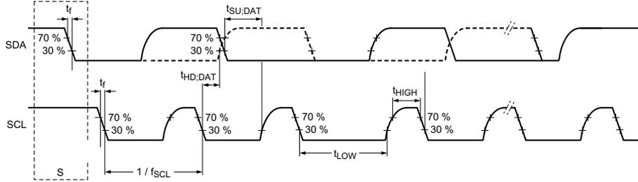
Fig 21. I<sup>2</sup>C interface timings
