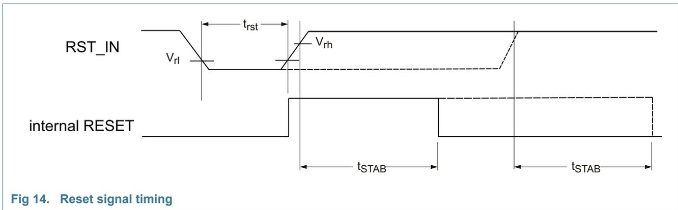
Fig 14. Reset signal timing
