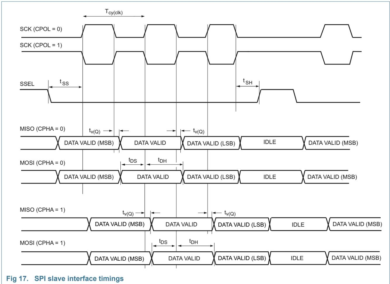
Fig 17. SPI slave interface timings
