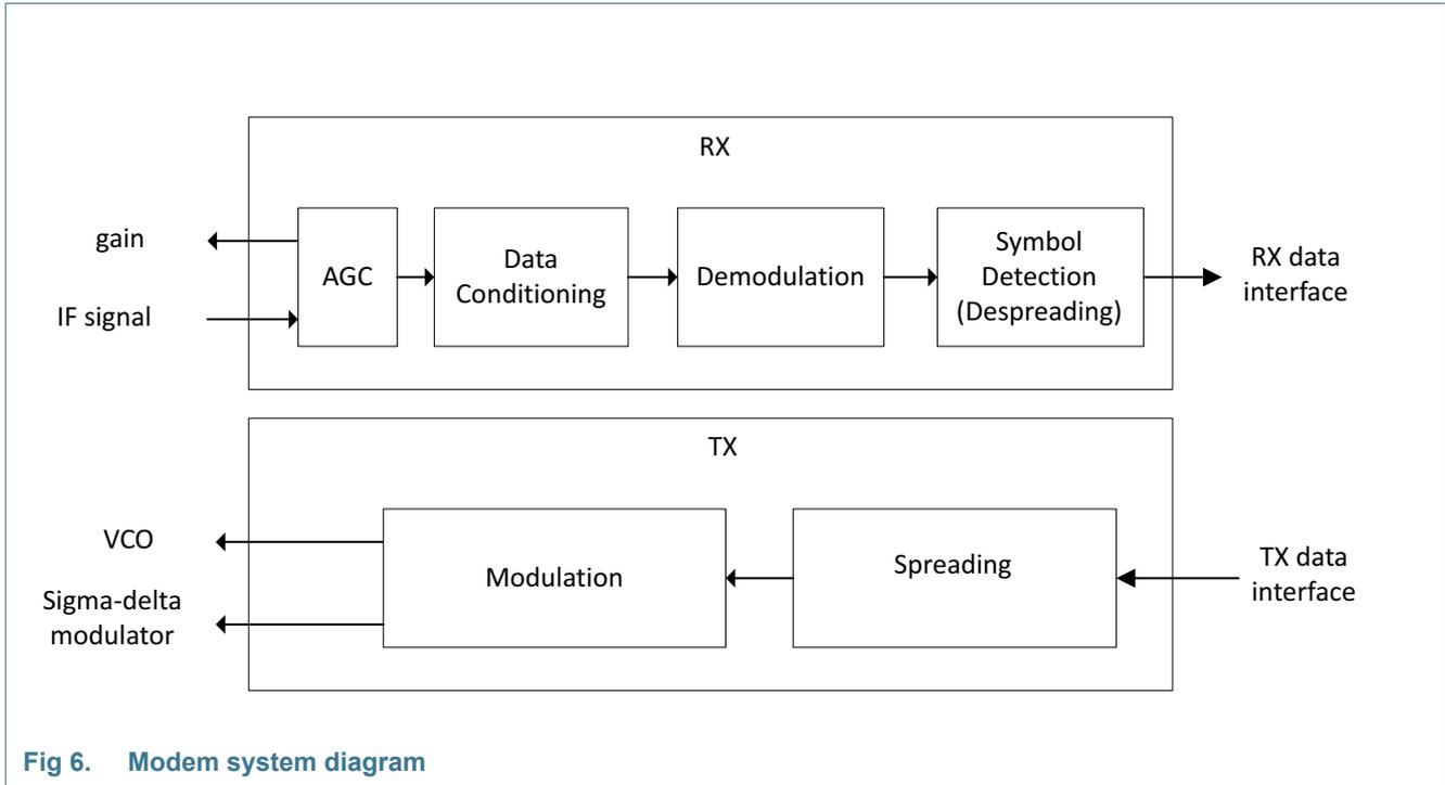
Fig 6. Modem system diagram
