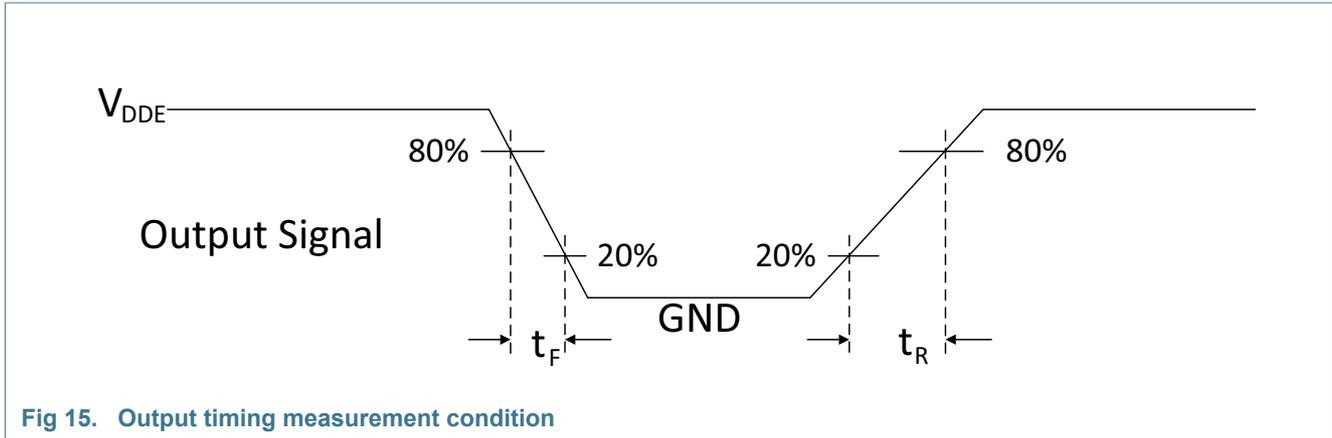
Fig 15. Output timing measurement condition
