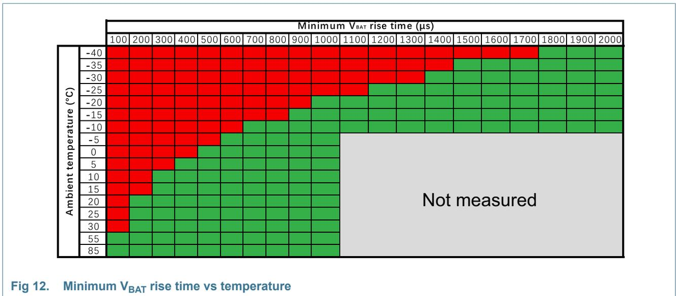
**Fig 12. Minimum V<sub>BAT</sub> rise time vs temperature**
