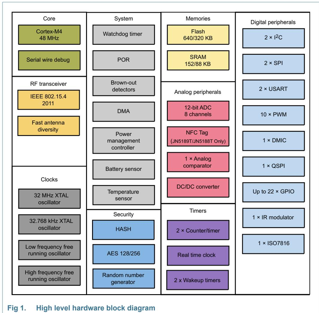
Fig 1. High level hardware block diagram
