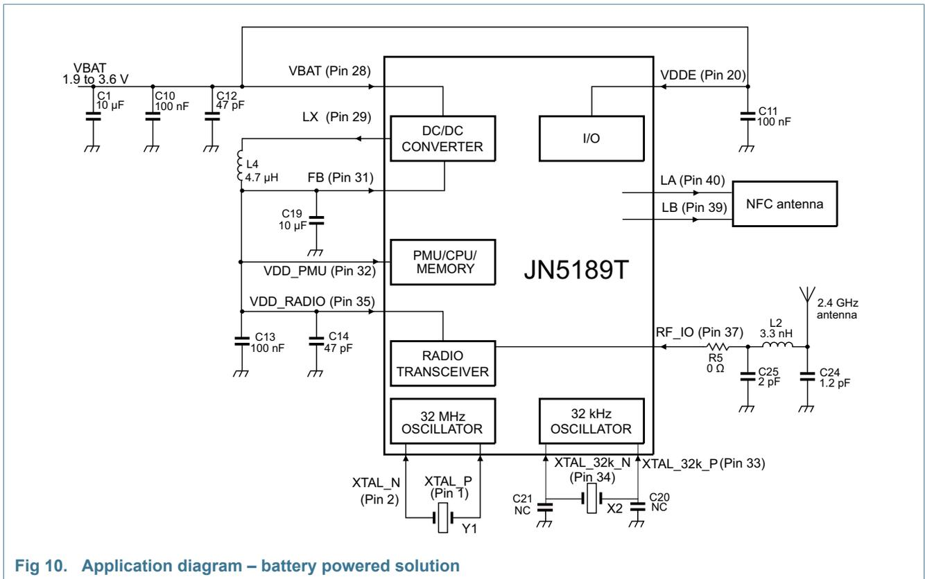
Fig 10. Application diagram – battery powered solution
