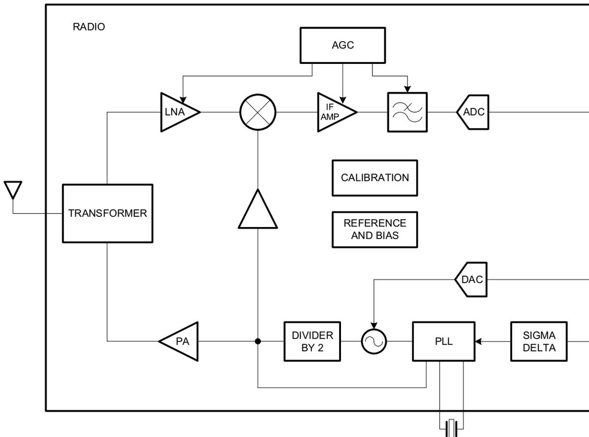
Fig 5. Radio architecture
