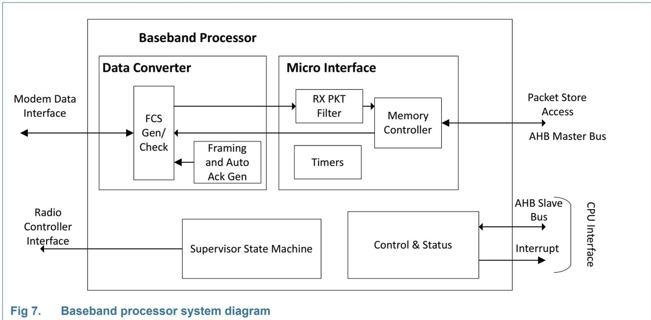
Fig 7. Baseband processor system diagram
