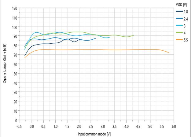
**Figure 49-9. Open Loop Gain at V<sub>CM</sub> = V<sub>DD</sub>/2 over V<sub>DD</sub> and Temperature**
