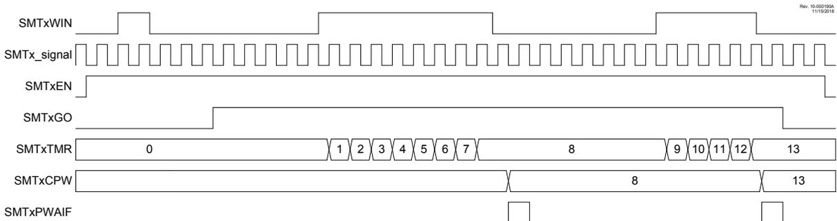
**Figure 27-20. Gated Counter Mode, Single Acquisition Timing Diagram**
