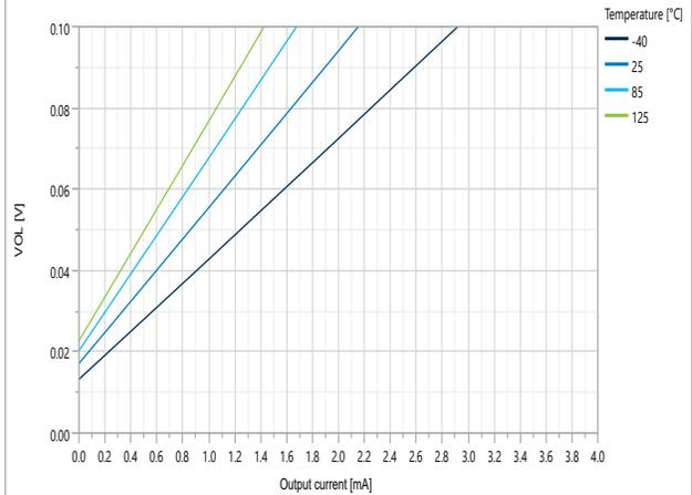
**Figure 49-15.  $V_{OL}$  at 5V over Temperature and Load Current**
