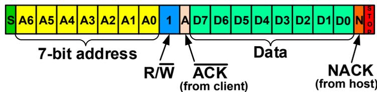
Figure 36-24. 7-Bit Host Read Diagram (from a specific memory/register location)
