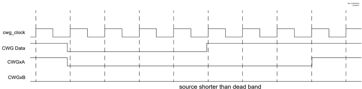
The CWGxDBF register value is double-buffered. When EN = 0, the buffer is loaded when CWGxDBF is written. When EN = 1, the buffer will be loaded at the rising edge following the first falling edge of the data input after the LD bit is set.
