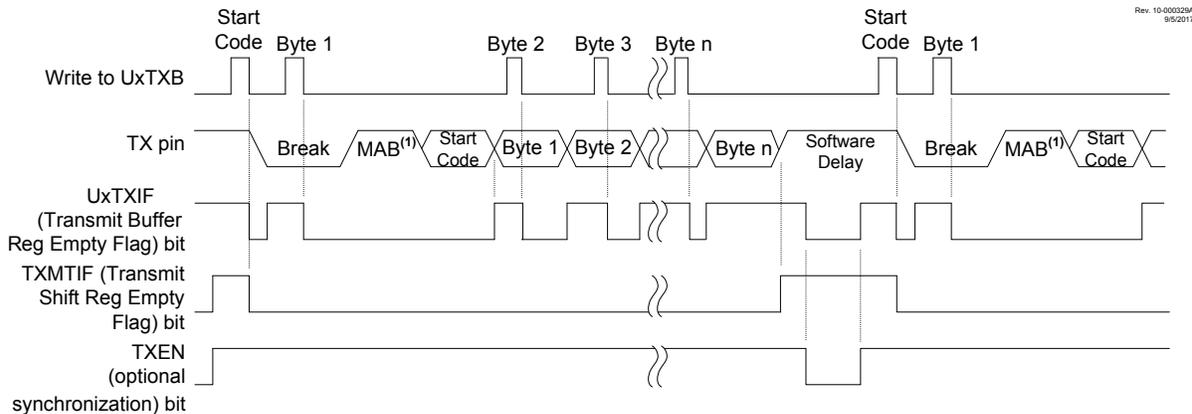
Software sends the Start Code and the ‘n’ data bytes by writing the UxTXB register with each byte to be sent in the desired order. A UxTXIF value of ‘1’ indicates when the UxTXB is ready to accept the next byte.
