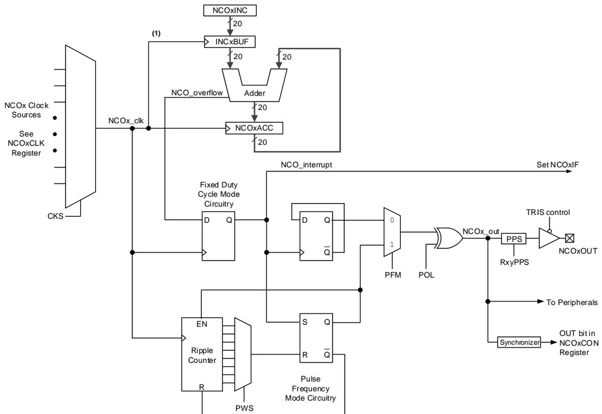
**Note 1:** The increment registers are double-buffered to allow for value changes to be made without first disabling the NCO module. The full increment value is loaded into the buffer registers on the second rising edge of the NCOx\_clk signal that occurs immediately after a write to the NCOxINCL register. The buffers are not user-accessible and are shown here for reference.
