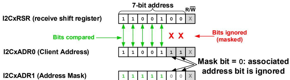
In 10-bit Address mode, I2CxADR0 and I2CxADR1, and I2CxADR2 and I2CxADR3 are combined to create two 10-bit addresses. I2CxADR0 and I2CxADR2 hold the lower eight bits of the address, while I2CxADR1 and I2CxADR3 hold the upper two bits of the address, the  $R/\bar{W}$  bit, and the five-digit '11110' code assigned to the five Most Significant bits of the high address byte.
