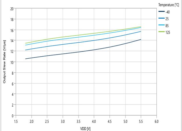
**Figure 49-11. Slew Rate Rise Time over V<sub>DD</sub> and Temperature**
