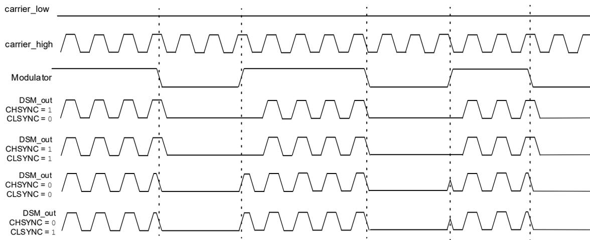
**Figure 33-3. No Synchronization (CHSYNC = 0, CLSYNC = 0)**
