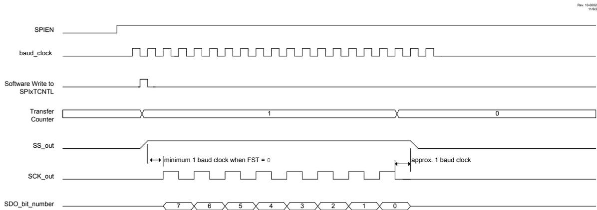
**Notes:** 1. *SDO bit number* illustrates the transmitted bit number, and is not intended to imply *SDO\_out* tristate operation.
