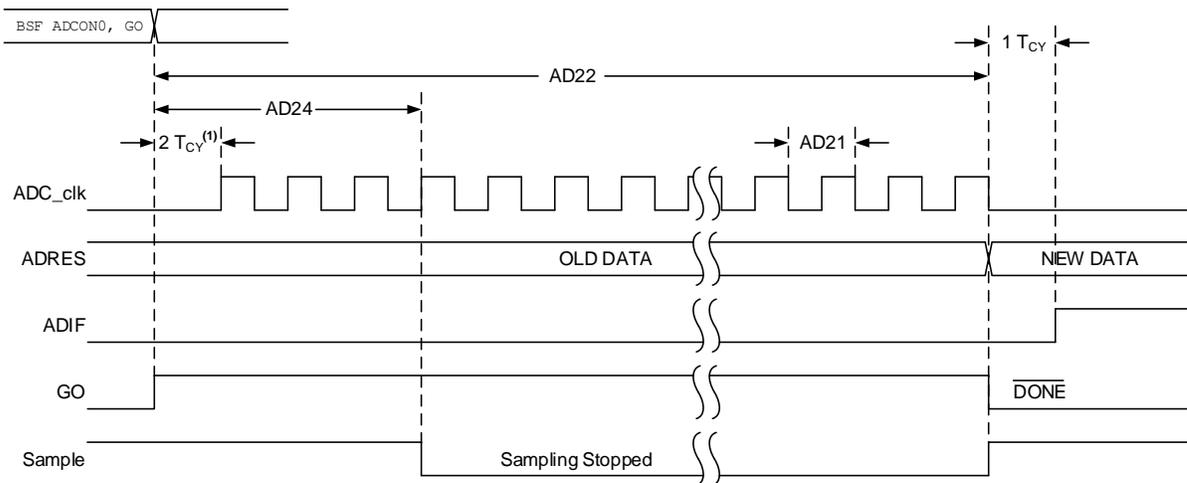
**Note 1:** If the ADC clock source is selected as ADCRC, a time of 1 T<sub>cy</sub> is added before the ADC clock starts. This allows the SLEEP instruction to be executed, if any.
