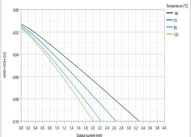
**Figure 49-13.  $V_{OH}$  at 5V over Temperature and Load Current**
