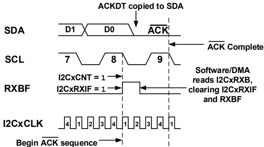
Figure 36-34. Not Acknowledge (NACK) Sequence Timing
