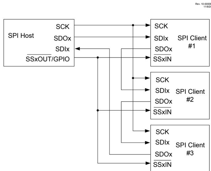
**Figure 35-13. SPI Daisy-Chain Connection with Chained SCK**
