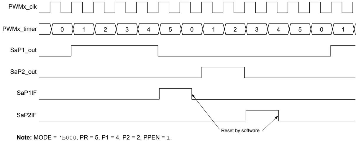
**Figure 30-14. Right Aligned Push-Pull Mode Timing Diagram**
