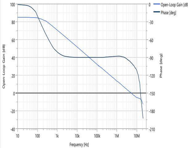
**Figure 49-8. Open Loop Gain at 25°C over V<sub>DD</sub> and V<sub>CM</sub>**
