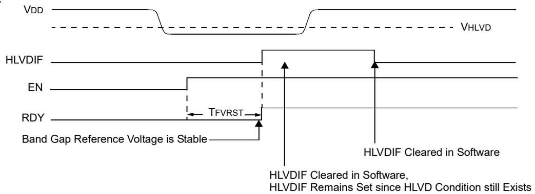
Figure 37-3. High-Voltage Detect Operation (INTH = 1)
