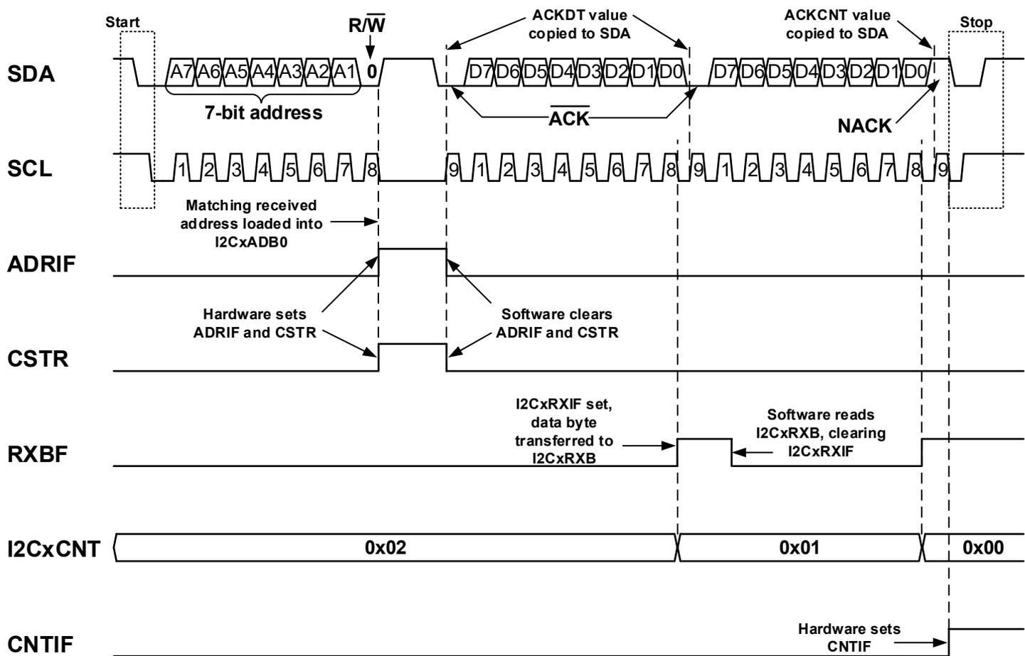
Figure 36-18. 7-Bit Client Mode Reception (ACKTIE = 1)
