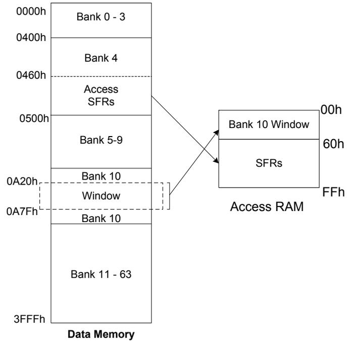
Remapping of the Access Bank applies only to operations using the Indexed Literal Offset mode. Operations that use the BSR (Access RAM bit is '1') will continue to use Direct Addressing as before.
