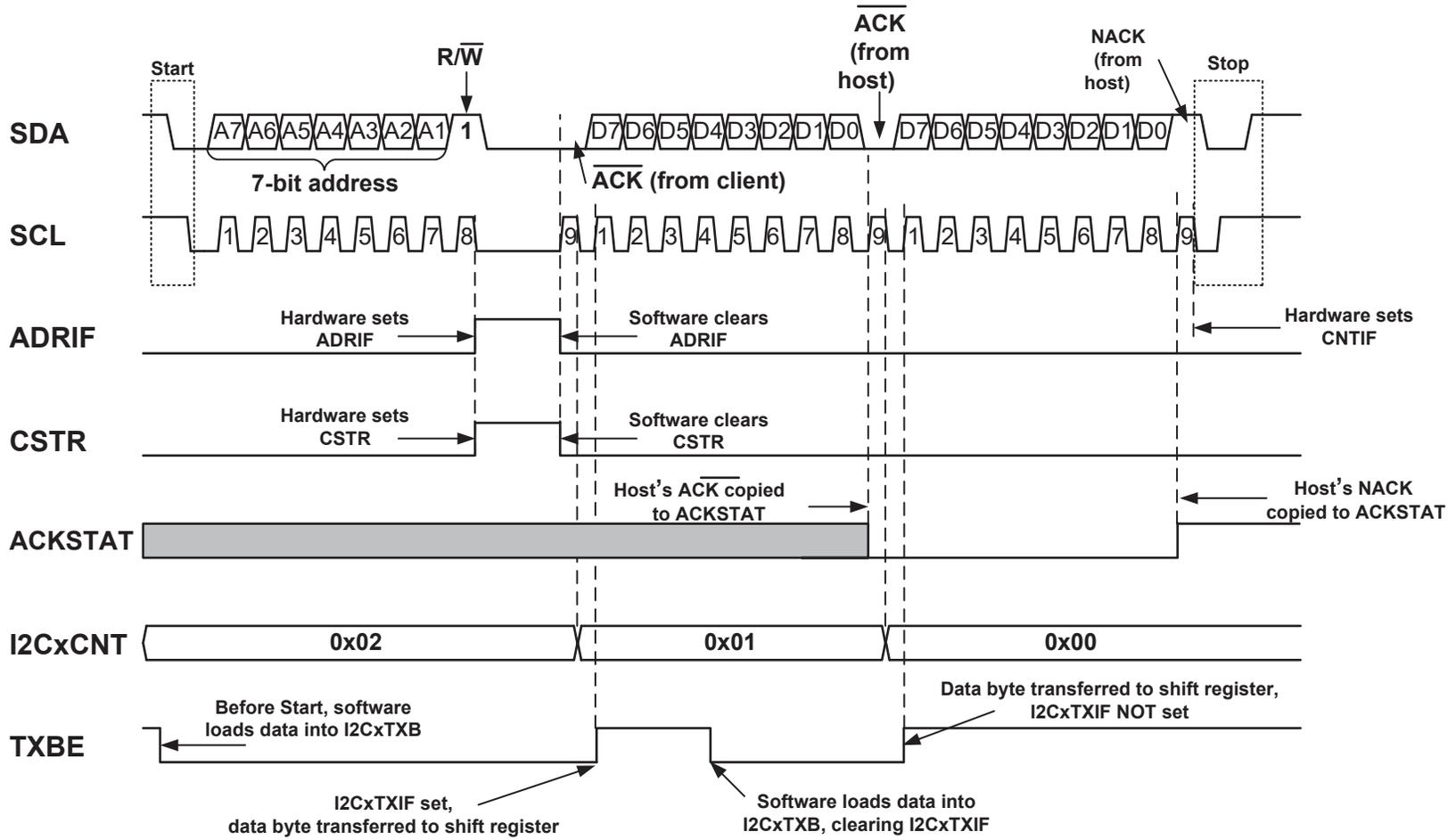
Figure 36-15. 7-Bit Client Mode Transmission (ACKTIE = 1)
