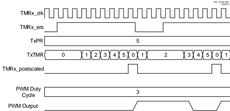
26.8.4 Level Triggered Hardware Limit Mode
