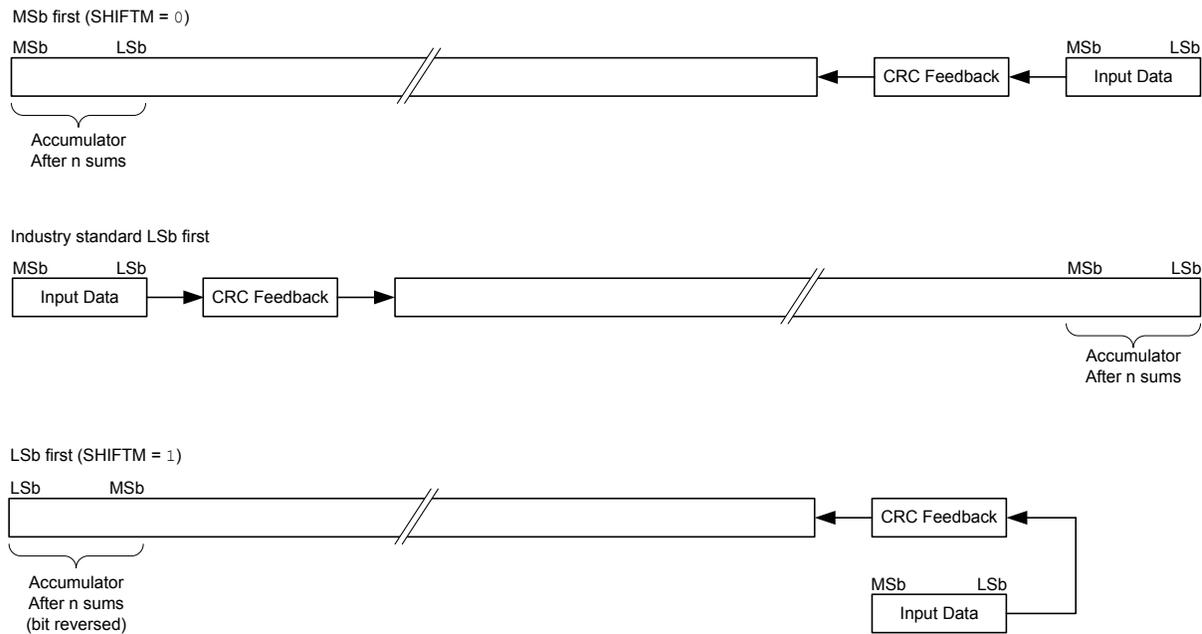
When the SHIFTM bit is not set, data will be shifted into the CRC, MSb first and the result will be big-endian. When the SHIFTM bit is set, data will be shifted into the accumulator in the reversed order (LSb first) and the result will be little-endian. The CRC module can be seeded with an initial value by setting the CRCOUT registers to the appropriate value before beginning the CRC process.
