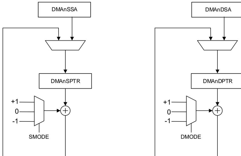
The DMA can initiate data transfers from the PFM, Data EEPROM or SFR/GPR space. The **SMR** bits are used to select the type of memory being pointed to by the Source Address Pointer. The SMR bits are required because the PFM and SFR/GPR spaces have overlapping addresses that do not allow the specified address to uniquely define the memory location to be accessed.
