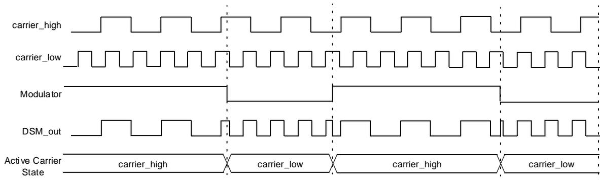
**Figure 33-4. Carrier High Synchronization (CHSYNC = 1, CLSYNC = 0)**
