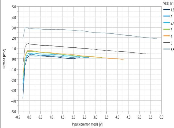
Figure 49-2. Input Offset Voltage at 25°C over  $V_{CM}$  and  $V_{DD}$  (CPON = 1)
