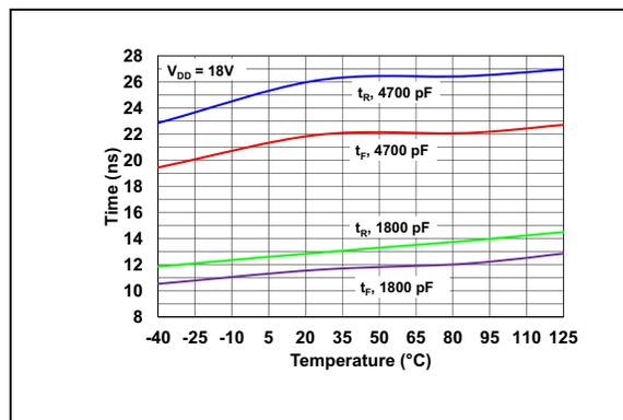
**FIGURE 2-5:** Rise and Fall Time vs. Temperature.
