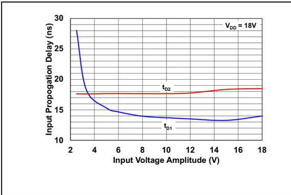
**FIGURE 2-8:** *Input Propagation Delay Time vs. Input Amplitude.*
