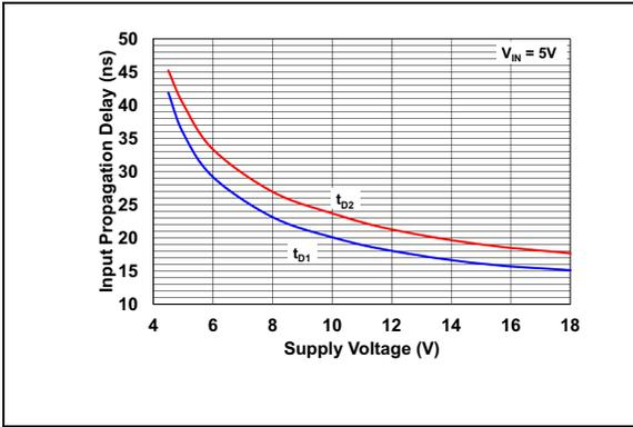
**FIGURE 2-7:** *Input Propagation Delay vs. Supply Voltage.*
