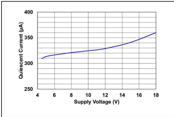
**FIGURE 2-13:** Quiescent Supply Current vs. Supply Voltage.
