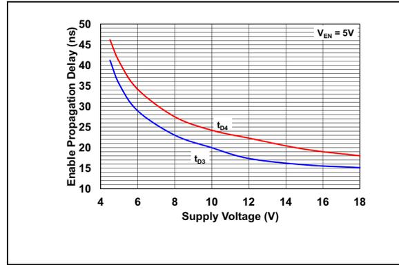
**FIGURE 2-10:** *Enable Propagation Delay vs. Supply Voltage.*
