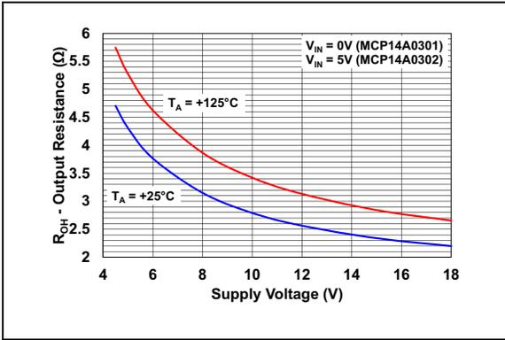
**FIGURE 2-19:** Output Resistance (Output High) vs. Supply Voltage.
