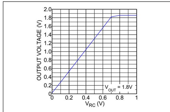
**FIGURE 2-12:** Output Voltage vs. Ramp Control Voltage.
