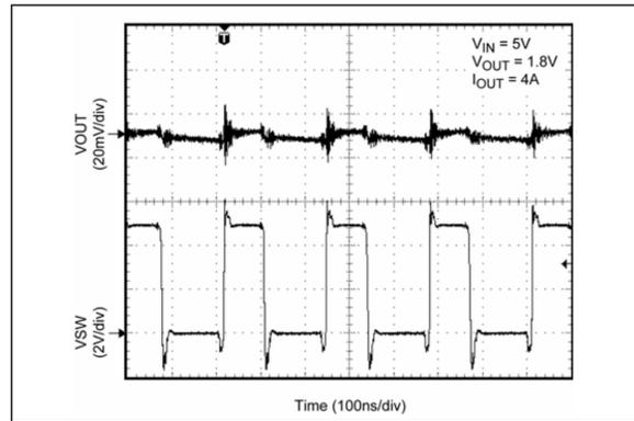
**FIGURE 2-24:** Output Noise and Ripple.
