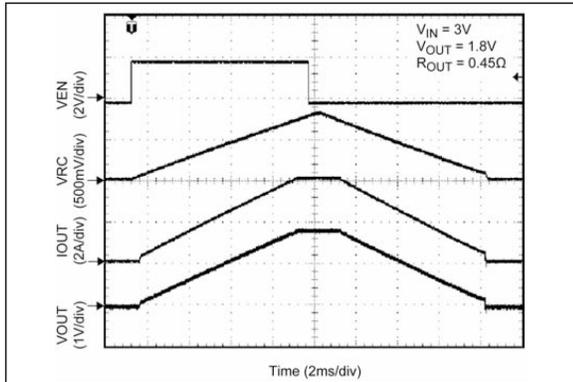
**FIGURE 2-19:** Start-Up/Shutdown ( $C_{RC} = 10 \text{ nF}$ ).
