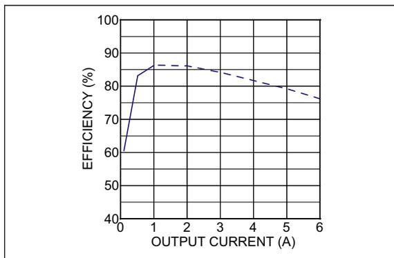
**FIGURE 5-1:** Efficiency 3.6V to 1.8V,  $L = 470 \text{ nH}$ .
