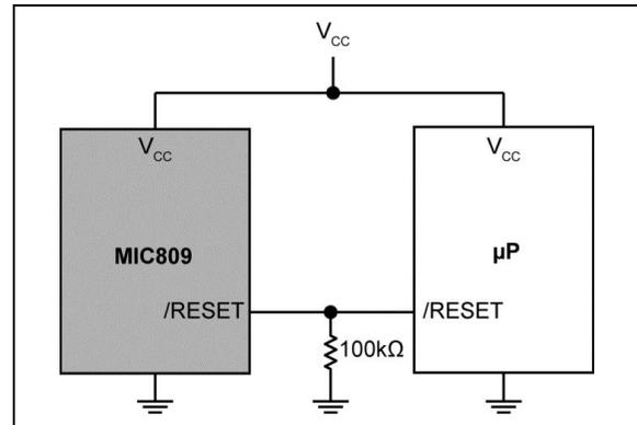
**FIGURE 3-1:** Reset Valid to  $V_{CC} = 0V$ .
