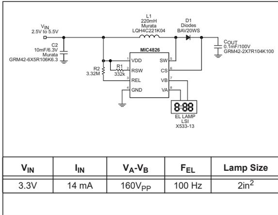
**FIGURE 5-3:** 100 Hz EL Driver for 2in<sup>2</sup> Lamp.
