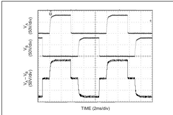
**FIGURE 5-4:** Typical Characteristics for EL Driver for 2in<sup>2</sup> Lamp with  $C_S = 0.1 \mu\text{F}$ .
