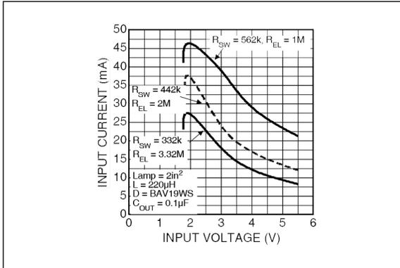
**FIGURE 2-1:** Total Input Current vs. Input Voltage.
