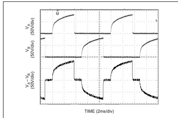
**FIGURE 5-6:** Typical Characteristics for EL Driver for 2in<sup>2</sup> Lamp with 560  $\mu\text{H}$  Inductor.
