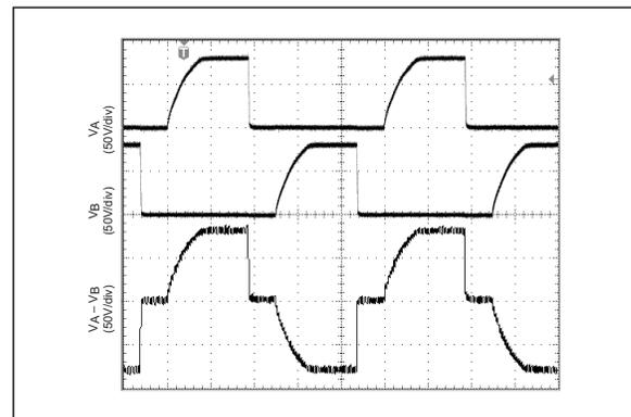
**FIGURE 5-2:** Typical Characteristics for 100 Hz EL Driver for 3in<sup>2</sup> Lamp.
