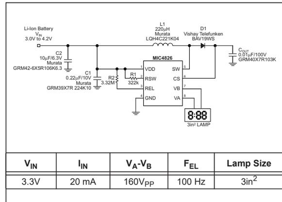
**FIGURE 5-1:** 100 Hz EL Driver for 3in<sup>2</sup> Lamp.
