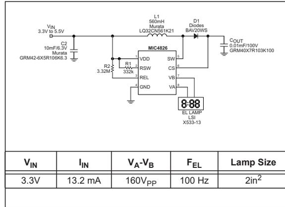
**FIGURE 5-5:** EL Driver for 2in<sup>2</sup> Lamp with 560  $\mu\text{F}$ .
