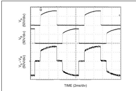
**FIGURE 5-8:** Typical Characteristics for Split Power Supplies Applications.
