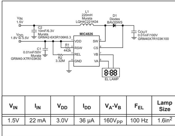
**FIGURE 5-7:** Typical for Split Power Supplies Applications.
