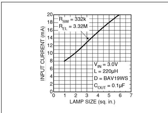
**FIGURE 2-15:** Total Input Current vs. Lamp Size.
