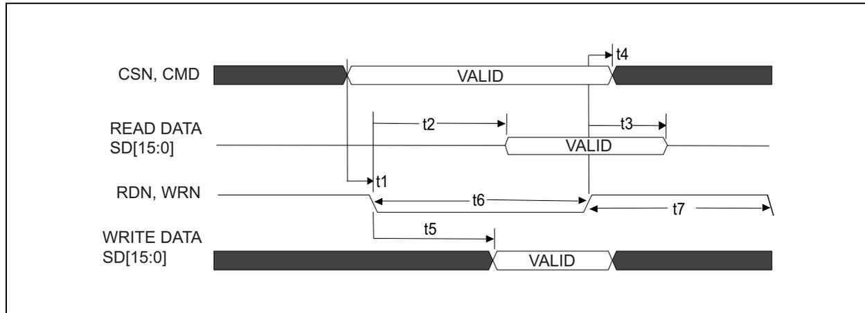
**TABLE 7-1: HOST INTERFACE READ/WRITE TIMING PARAMETERS**
