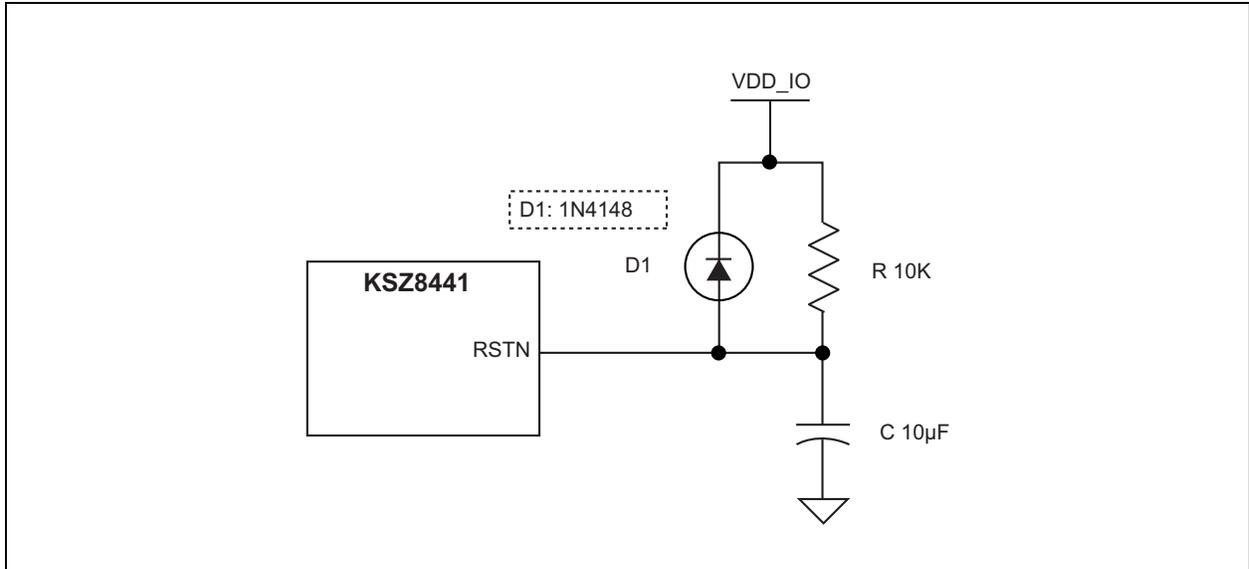
The following reset circuit is recommended for applications where reset is driven by another device (e.g., CPU or FPGA). At POR, R, C, and D1 provide the necessary ramp rise time to reset the KSZ8441 device. The RST\_OUT\_N from CPU/FPGA provides the warm reset after power-up.
