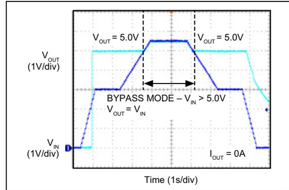
**FIGURE 2-22:** Bypass Mode.
