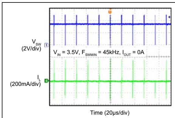
**FIGURE 2-20:** Minimum Switching.
