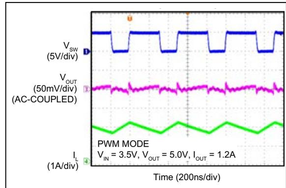
**FIGURE 2-17:** Output Ripple (PWM Mode).
