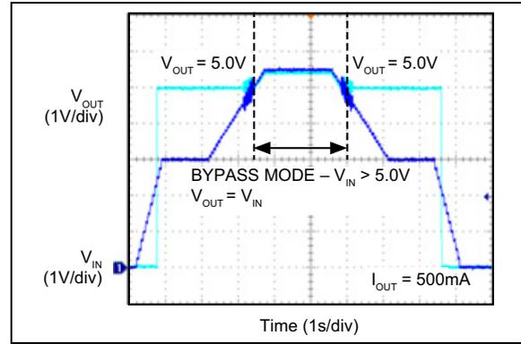
**FIGURE 2-23:** Bypass Mode.
