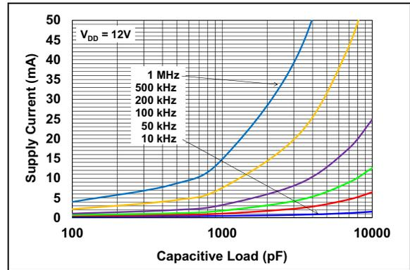
**FIGURE 2-22:** Supply Current vs. Capacitive Load ( $V_{DD} = 12\text{V}$ ).
