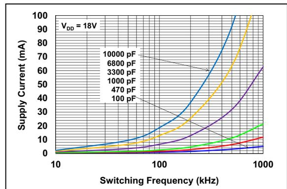
**FIGURE 2-24:** Supply Current vs. Frequency ( $V_{DD} = 18\text{V}$ ).
