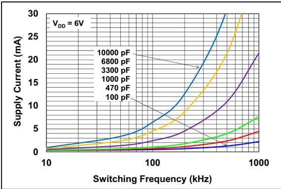
**FIGURE 2-26:** Supply Current vs. Frequency ( $V_{DD} = 6\text{V}$ ).
