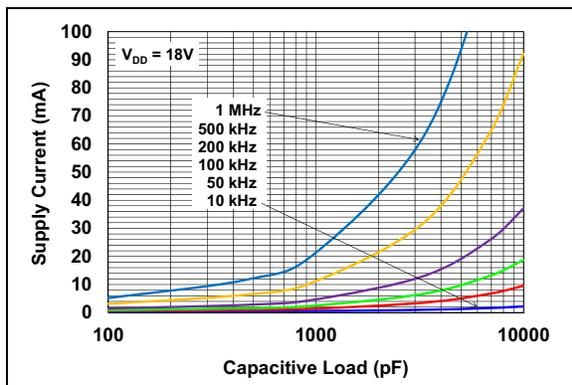
**FIGURE 2-21:** Supply Current vs. Capacitive Load ( $V_{DD} = 18\text{V}$ ).
