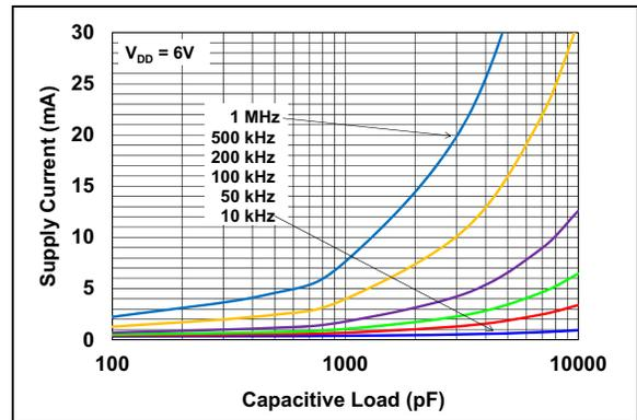
**FIGURE 2-23:** Supply Current vs. Capacitive Load ( $V_{DD} = 6\text{V}$ ).
