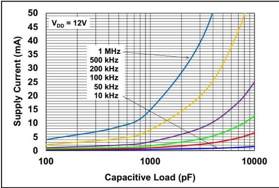
**FIGURE 2-25:** Supply Current vs. Frequency ( $V_{DD} = 12\text{V}$ ).
