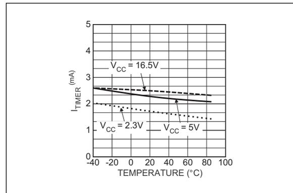
**FIGURE 2-5:** Overcurrent Timer (Off) Current vs. Temperature.
