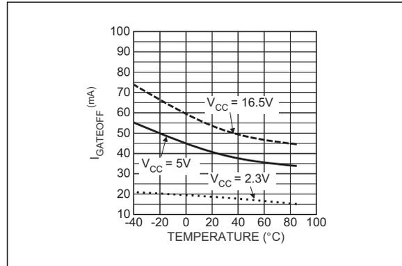
**FIGURE 2-10:** Gate Sink Current vs. Temperature.
