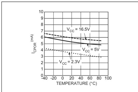
**FIGURE 2-3:** Power-On Reset Timer (Off) Current vs. Temperature.
