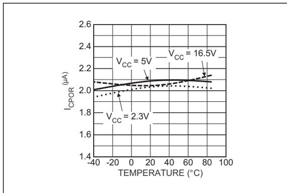
**FIGURE 2-2:** Power-On Reset Timer Current vs. Temperature.
