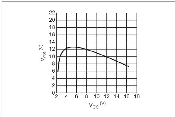
**FIGURE 2-9:** External Gate Drive vs.  $V_{CC}$ .
