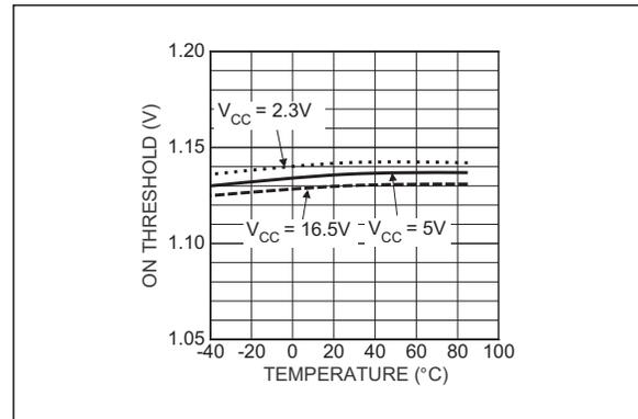
**FIGURE 2-17:** ON Pin Threshold (Falling) vs. Temperature.
