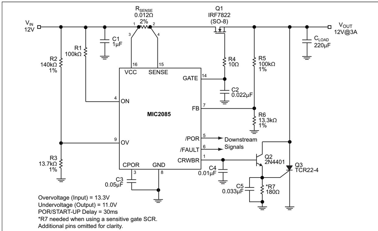
**FIGURE 5-1:** Undervoltage/Overvoltage Circuit.
