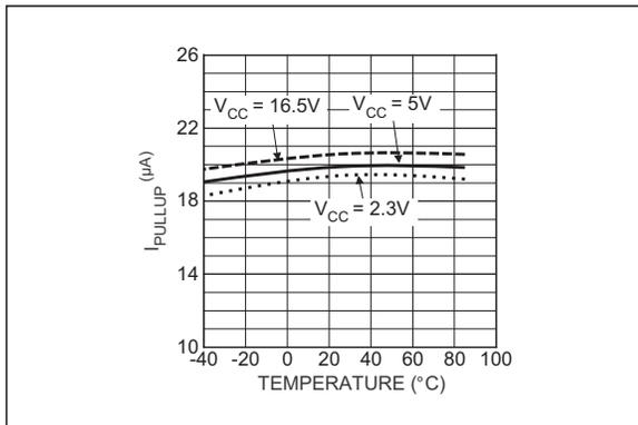
**FIGURE 2-21:** Output Signal Pull-Up Current vs. Temperature.
