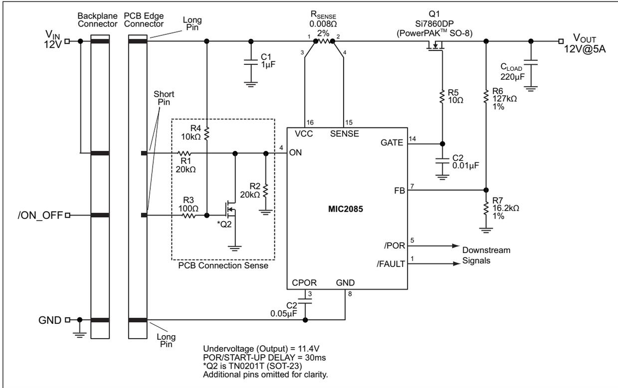
FIGURE 5-2: PCB Connection Sense with ON/OFF Control.
