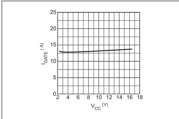
**FIGURE 2-7:** Gate Pull-Up Current vs  $V_{CC}$ .
