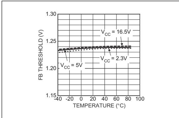
**FIGURE 2-19:** FB (Power Good) Threshold vs. Temperature.
