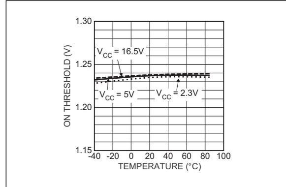
**FIGURE 2-16:** ON Pin Threshold (Rising) vs. Temperature.
