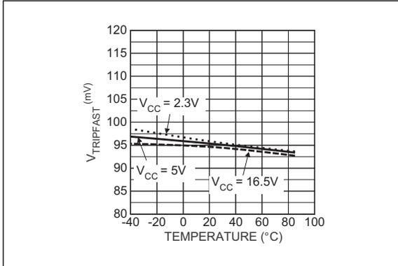
**FIGURE 2-13:** Current Limit Threshold (Fast Trip) vs. Temperature.
