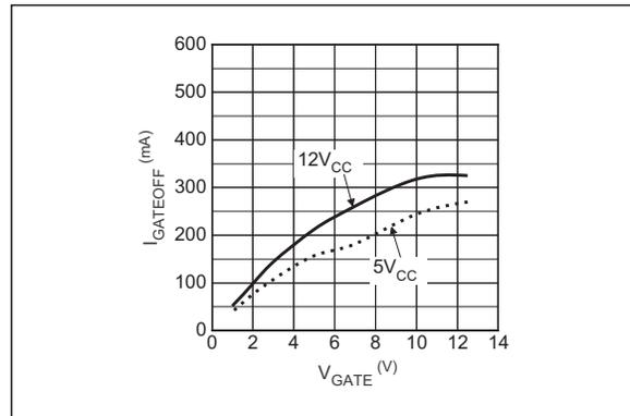
**FIGURE 2-11:** Gate Sink Current vs. Gate Voltage.
