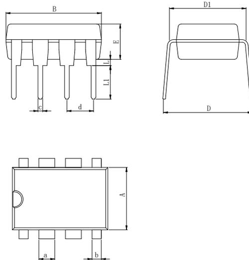
**Dimensions In Millimeters(DIP8)**
