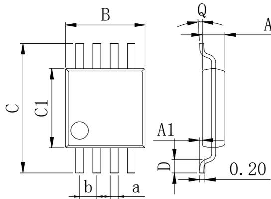
**Dimensions In Millimeters(MSOP8)**
