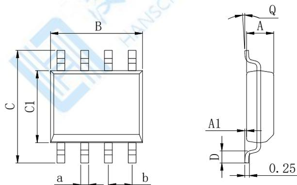
**Dimensions In Millimeters(SOP8)**
