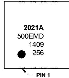
8-Lead SOIC (150 mil) (MCP2021A)
