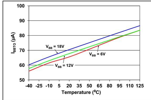
**FIGURE 2-6:** Typical  $I_{BBTQ}$  vs. Temperature – 3.3V.
