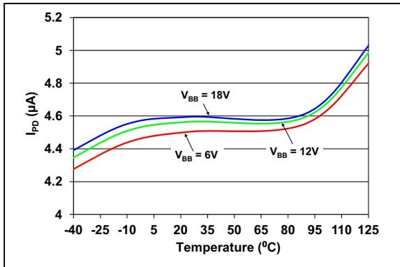
**FIGURE 2-4:** Typical  $I_{PD}$  vs. Temperature – 5.0V.
