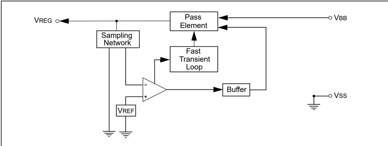
**FIGURE 1-5: VOLTAGE REGULATOR OUTPUT ON OVERCURRENT PROTECTION**
