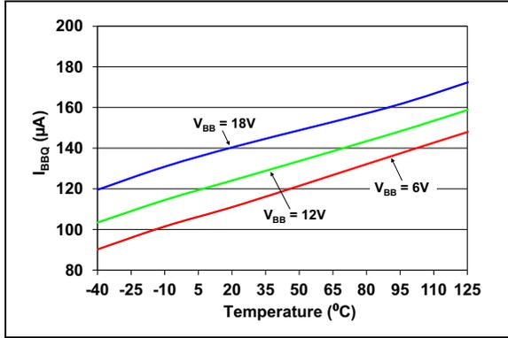
**FIGURE 2-2:** Typical  $I_{BBQ}$  vs. Temperature – 5.0V.
