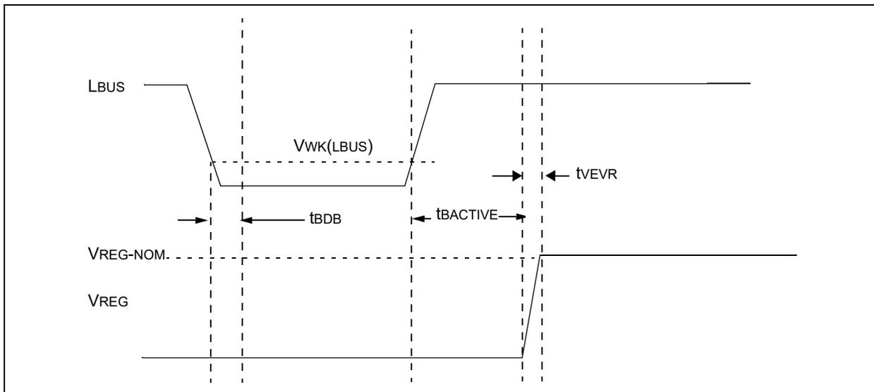
FIGURE 2-12: CS/LWAKE, REGULATOR AND RESET TIMING DIAGRAM
