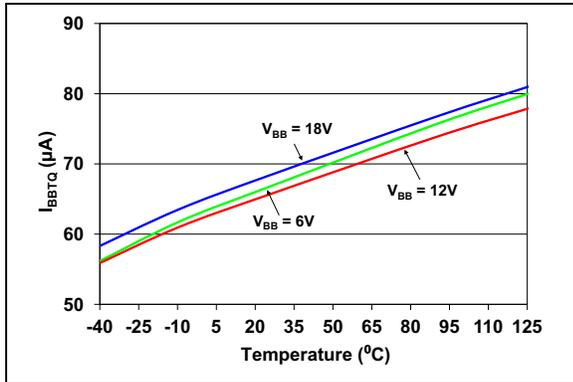
**FIGURE 2-3:** Typical  $I_{BBTQ}$  vs. Temperature – 5.0V.
