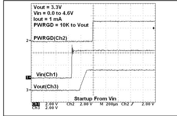
**FIGURE 2-27:** Power-up Timing.
