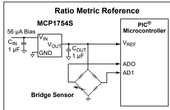
**FIGURE 5-2:** Using the MCP1754/MCP1754S as a Voltage Reference.
