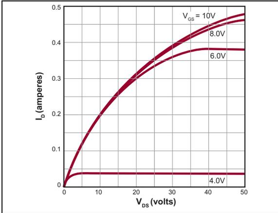
**FIGURE 2-1:** Output Characteristics.
