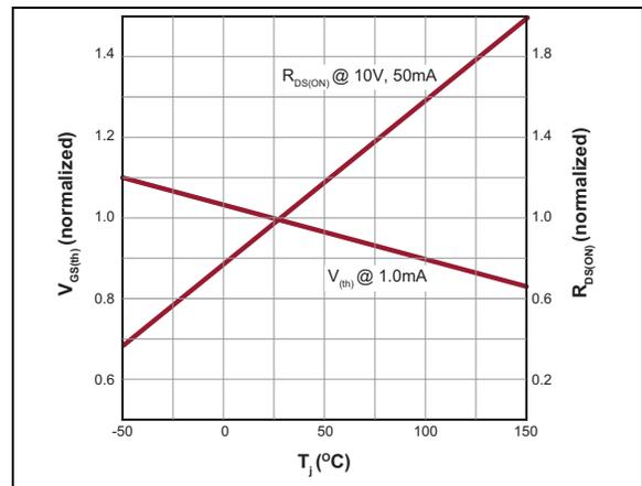
**FIGURE 2-11:**  $V_{(th)}$  and  $R_{DS}$  Variation with Temperature.
