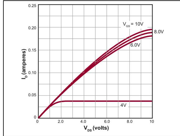
**FIGURE 2-4:** Saturation Characteristics.
