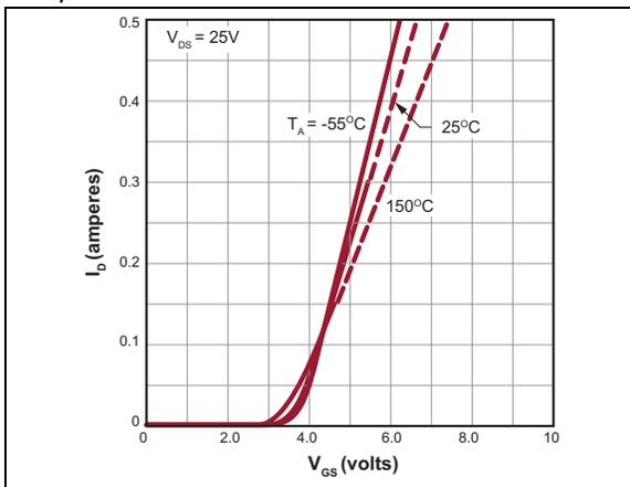
**FIGURE 2-8:** Transfer Characteristics.
