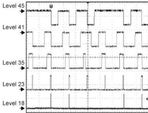
Figure 4. LED Current with Brightness Level Change
