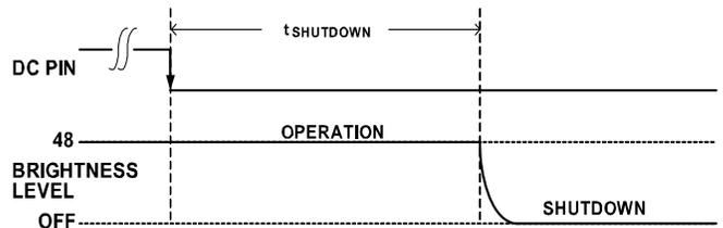
Figure 7. Shutdown Timing
