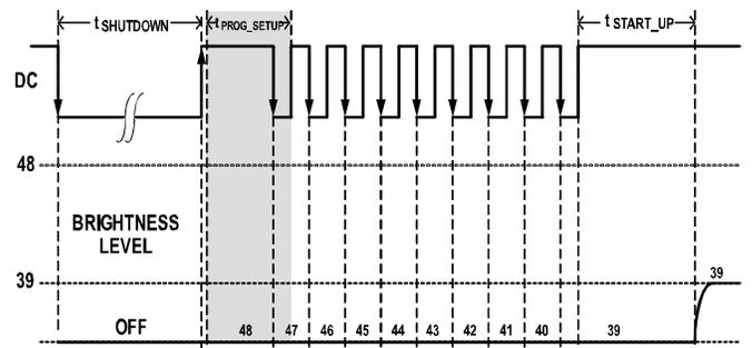
Figure 16. Presetting Timing
