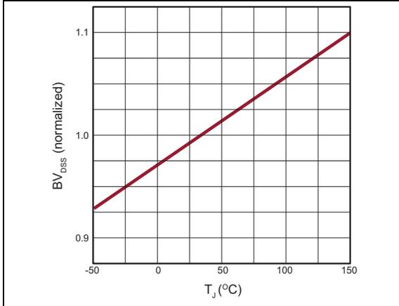
**FIGURE 2-7:**  $B_{V_{DS}}$  Variation with Temperature.
