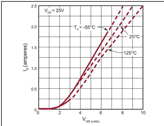
**FIGURE 2-8:** Transfer Characteristics.
