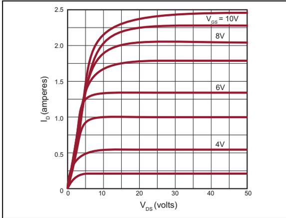
**FIGURE 2-1:** Output Characteristics.
