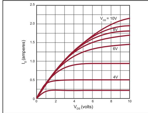
**FIGURE 2-4:** Saturation Characteristics.
