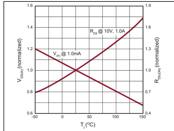
**FIGURE 2-11:**  $V_{GS(th)}$  and  $R_{DS}$  Variation with Temperature.
