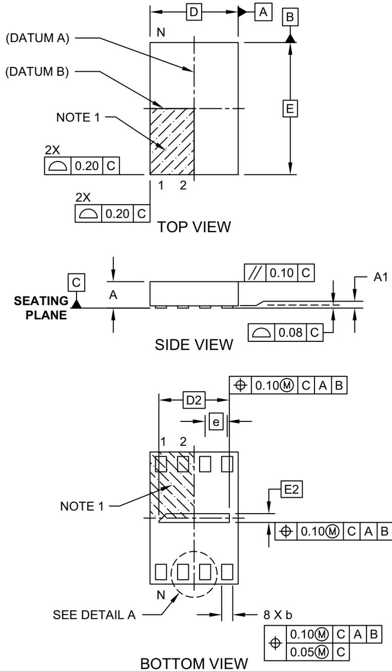
**8-Lead Plastic Ultra Thin Small Outline No Lead Package (PRX) - 2x3 mm Body [USON]
