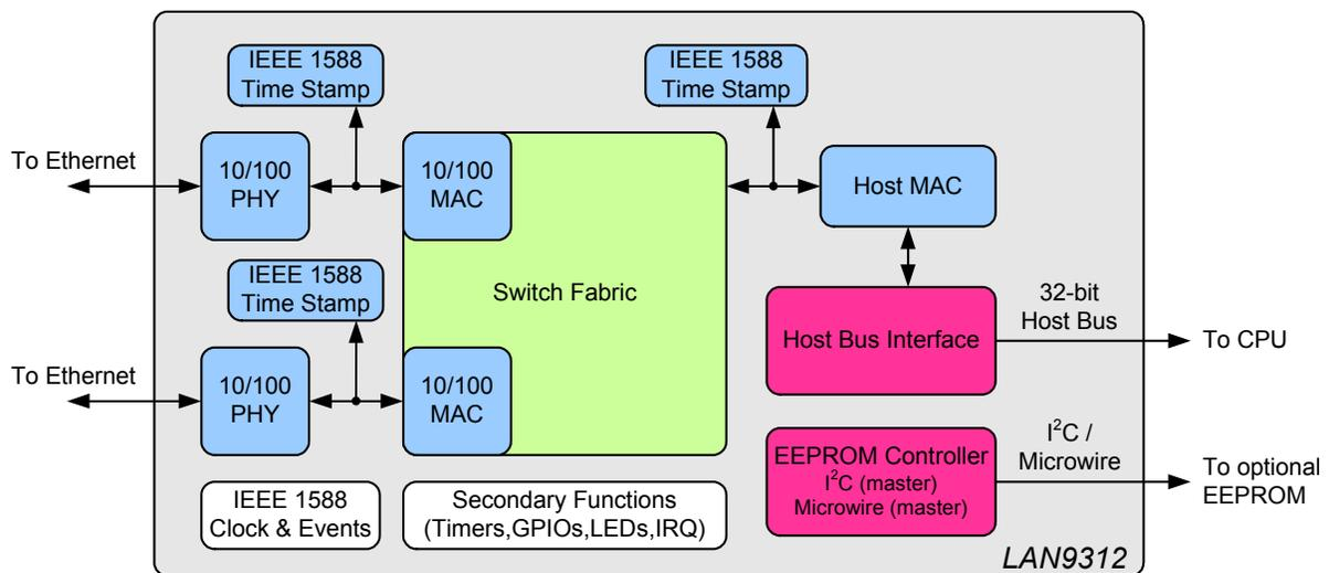
Figure 2 LAN9312 Internal Block Diagram
