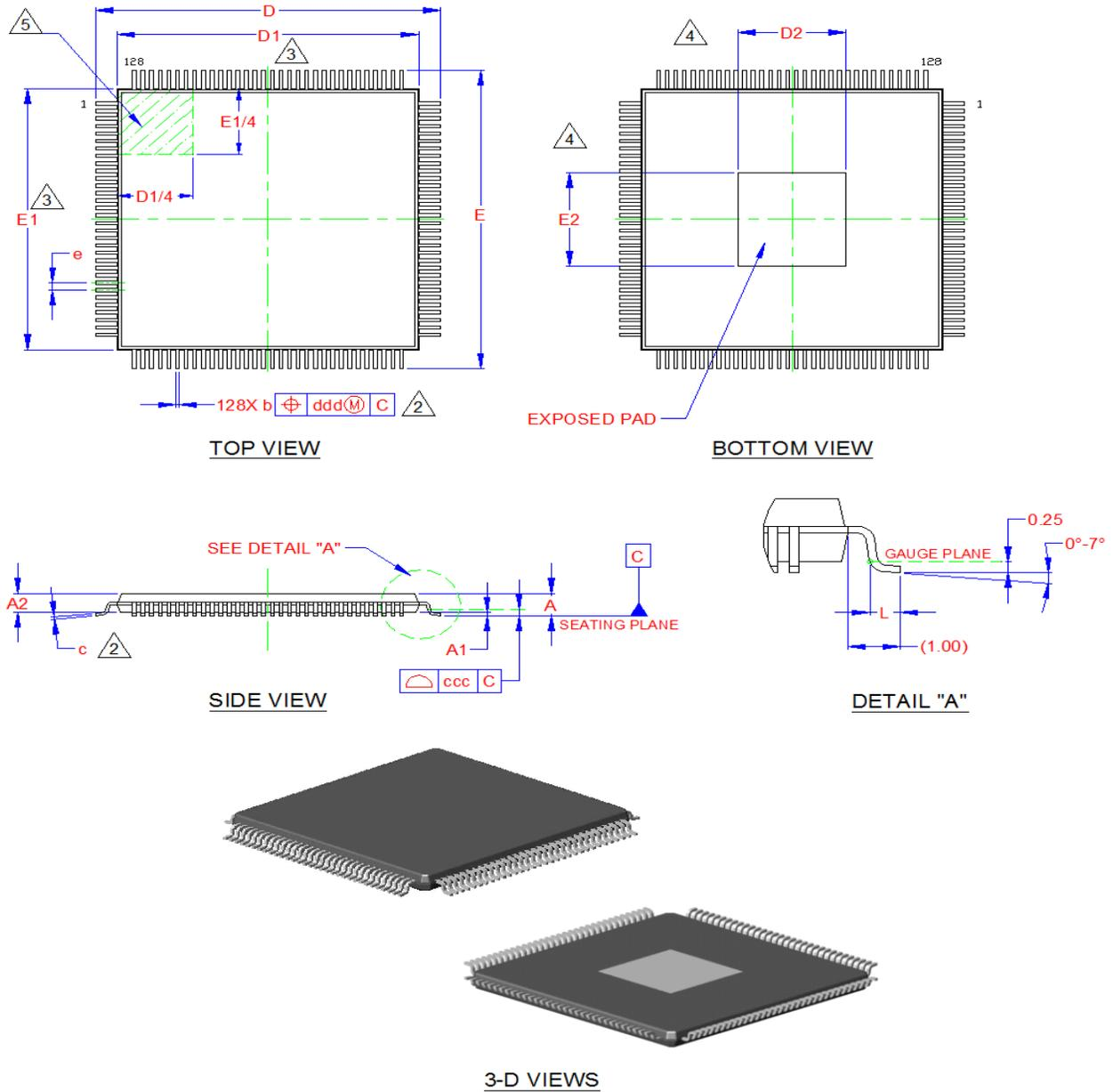
Figure 5 LAN9312 128-XVTQFP Package Definition
