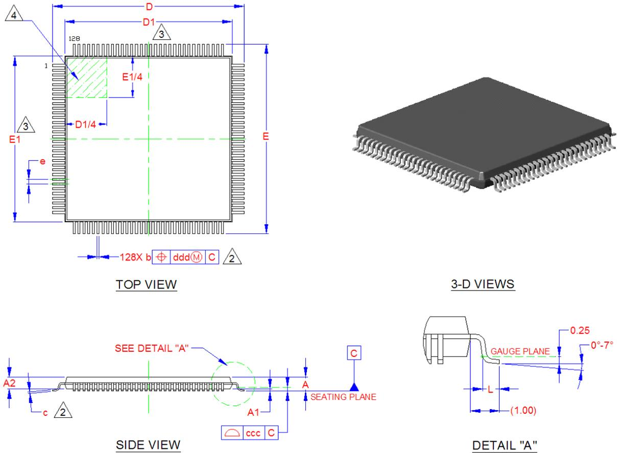
Figure 3 LAN9312 128-VTQFP Package Definition
