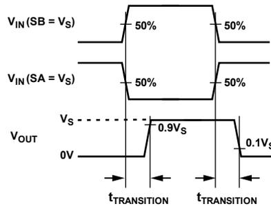
\*ALTERNATIVELY, SB CAN BE CONNECTED TO VS WITH SA CONNECTED TO GROUND.
