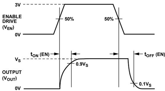
Figure 33. Enable Delay,  $t_{ON}(EN)$ ,  $t_{OFF}(EN)$  (LFCSP Only)
