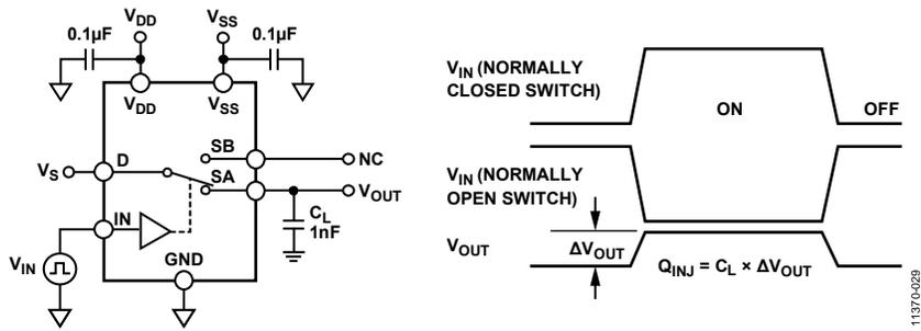
Figure 35. Charge Injection
