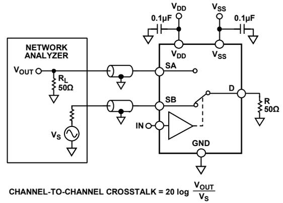
Figure 28. Channel-to-Channel Crosstalk
