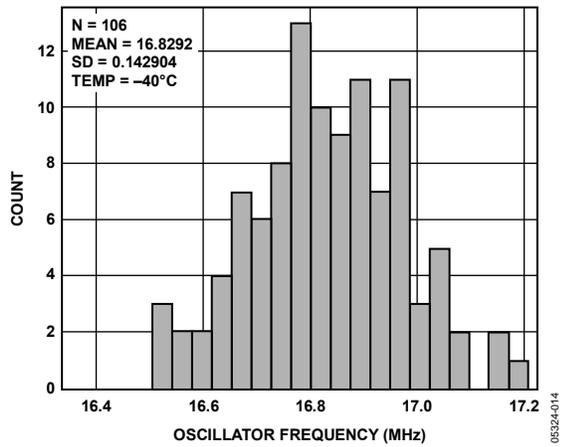
Figure 14. Frequency Distribution of Internal Oscillator at -40°C
