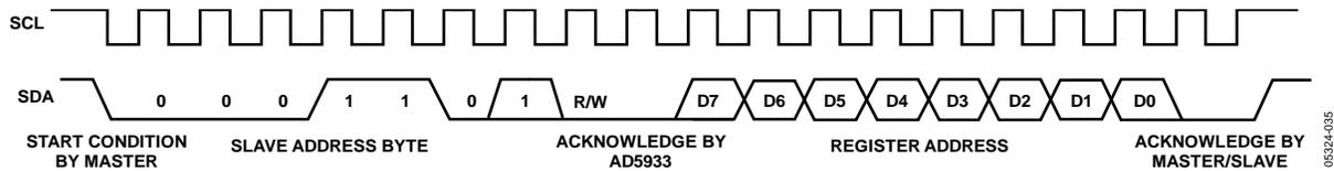
Figure 29. Timing Diagram
