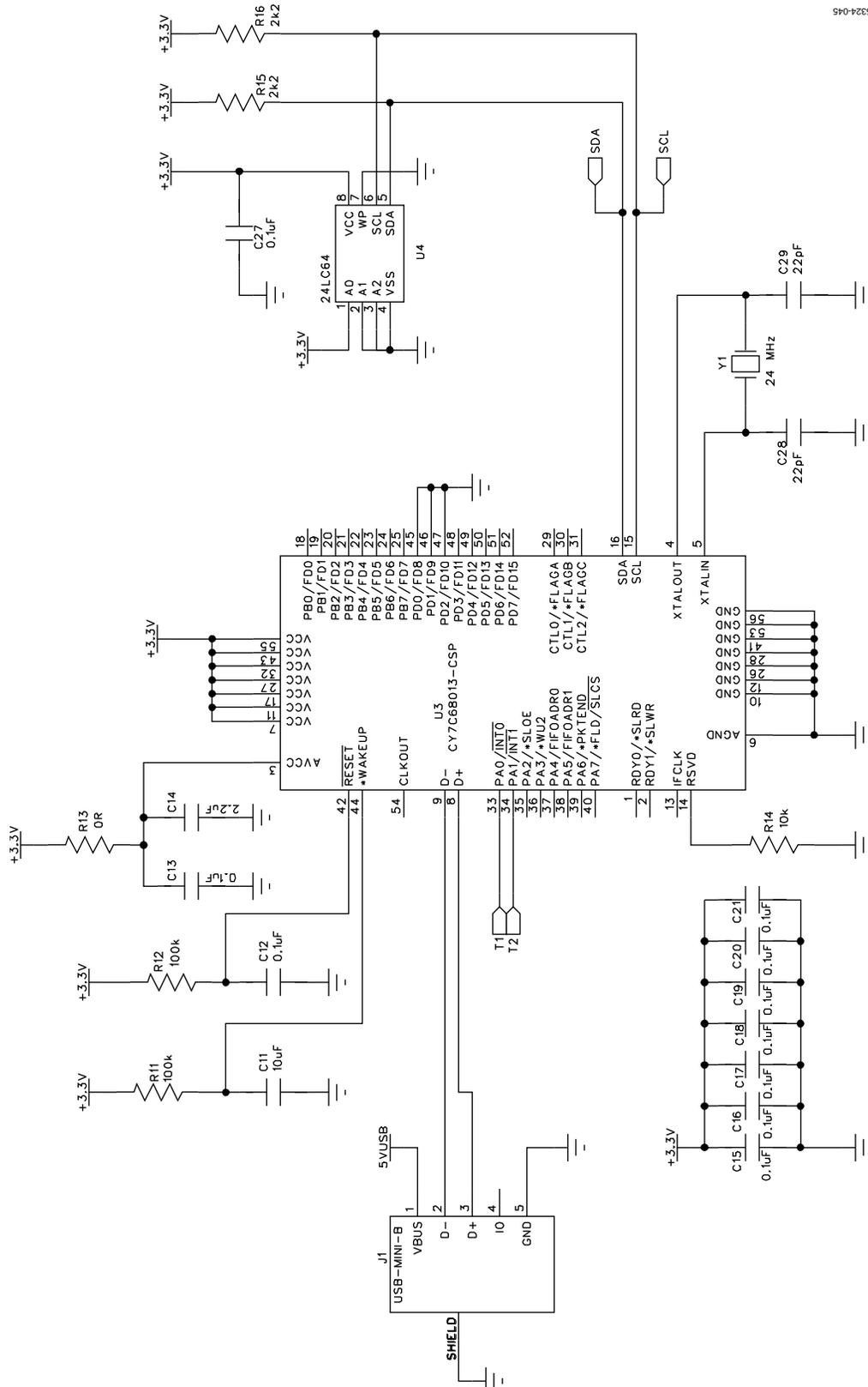
Figure 40. EVAL-AD5933EBZ Schematic
