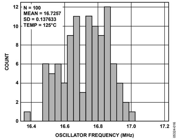
Figure 16. Frequency Distribution of Internal Oscillator at 125°C
