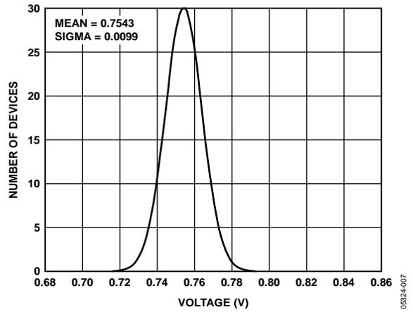
Figure 7. Range 2 DC Bias Distribution, VDD = 3.3 V
