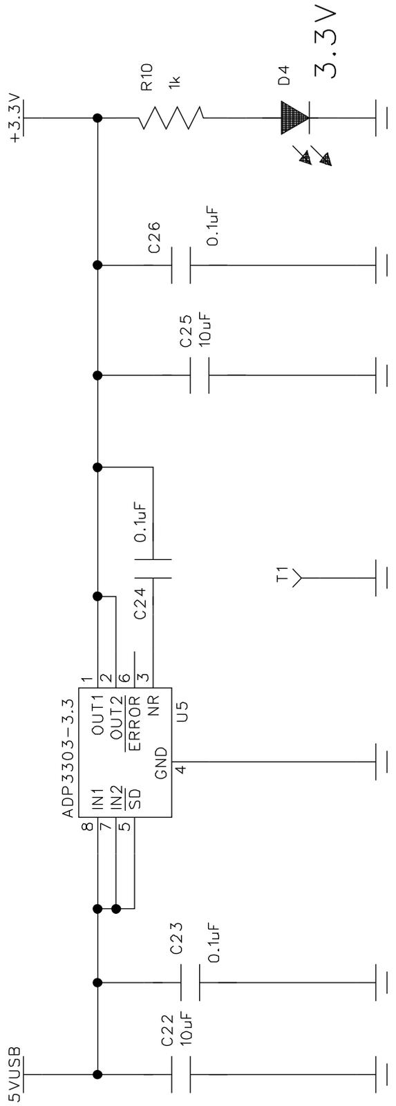
Figure 41. Linear Regulator on the EVAL-AD5933EB Evaluation Board
