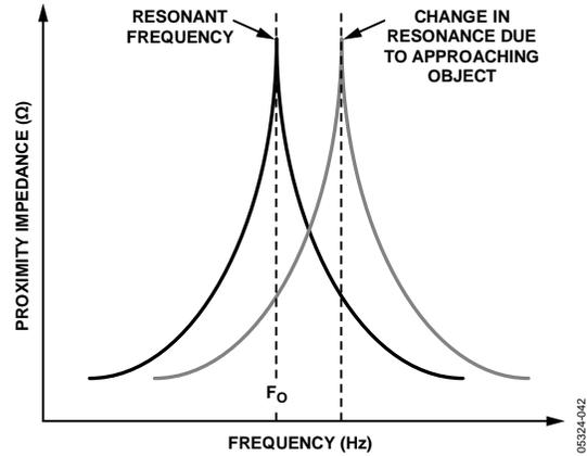
Figure 37. Detecting a Change in Resonant Frequency
