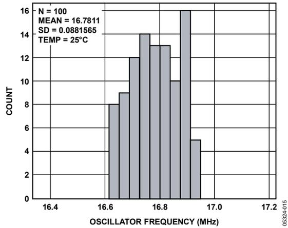
Figure 15. Frequency Distribution of Internal Oscillator at 25°C
