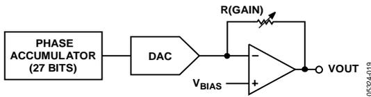
Figure 19. Transmit Stage
