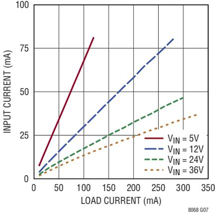
**Input Current vs Load Current,
