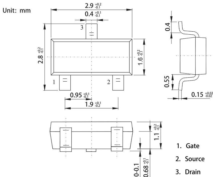
P-Channel Enhancement Mode Field Effect Transistor
