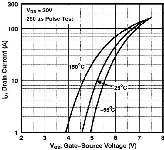
Figure 3. Transfer Characteristics
