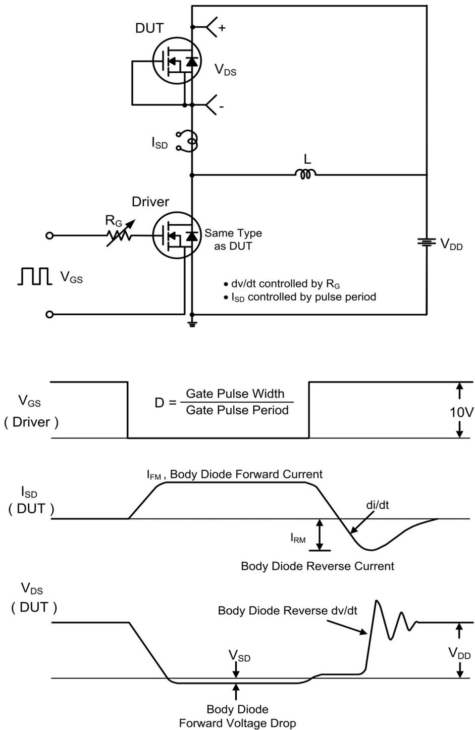
Figure 20. Peak Diode Recovery dv/dt Test Circuit & Waveforms
