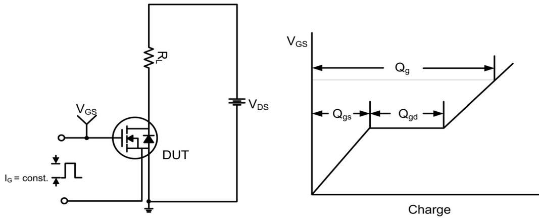
Figure 17. Gate Charge Test Circuit & Waveform
