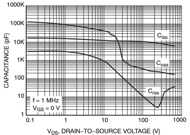
Figure 6. Capacitance Characteristics
