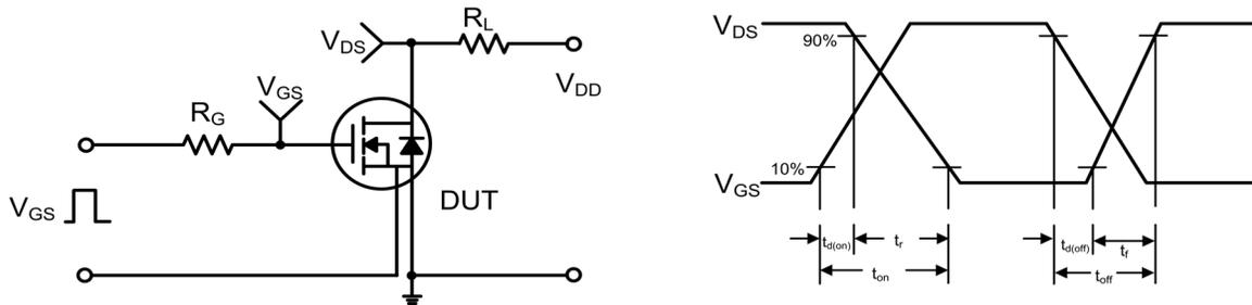
Figure 18. Resistive Switching Test Circuit & Waveforms
