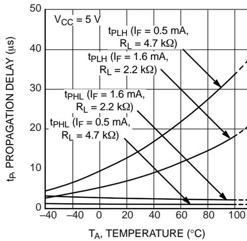
Figure 13. Propagation Delay vs. Temperature (6N138M / 6N139M Only)
