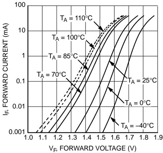
Figure 5. LED Forward Current vs. Forward Voltage
