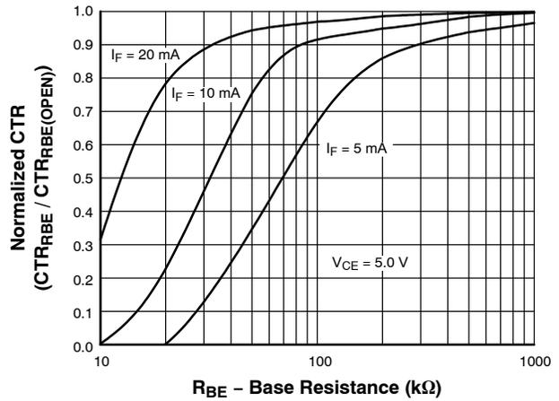
Figure 4. CTR vs. RBE (Unsaturated)
