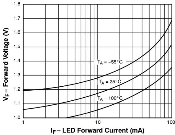
Figure 1. LED Forward Voltage vs. Forward Current
