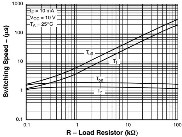
Figure 7. Switching Speed vs. Load Resistor
