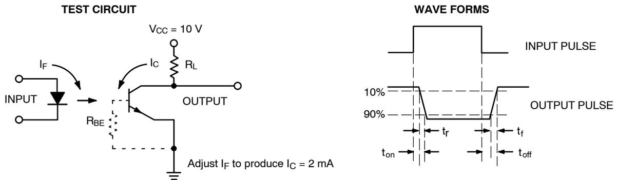
Figure 11. Switching Time Test Circuit and Waveforms
