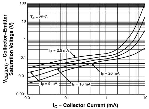
Figure 6. Collector-Emitter Saturation Voltage vs. Collector Current
