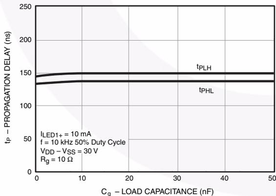
Figure 21. Propagation Delay ( $t_p$ ) vs. Load Capacitance ( $C_g$ )
