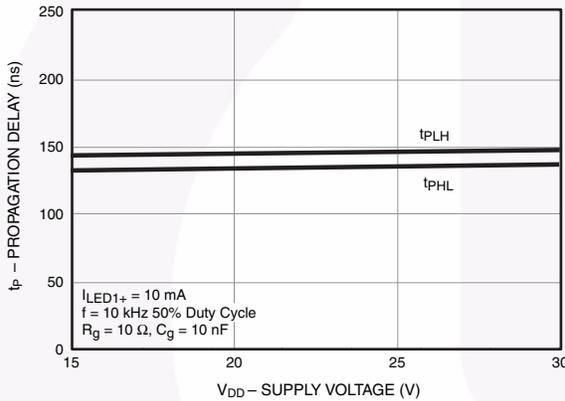
Figure 19. Propagation Delay ( $t_p$ ) vs. Supply Voltage ( $V_{DD}$ )
