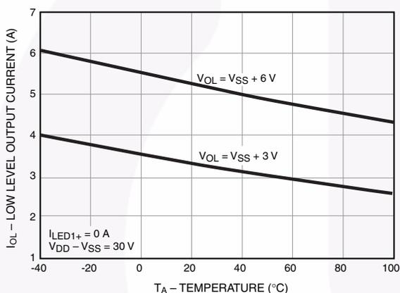
Figure 7. Low Level Output Current ( $I_{OL}$ ) vs. Temperature
