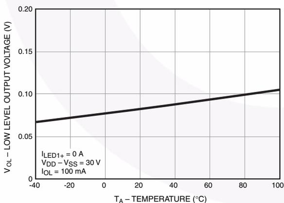
Figure 9. Low Level Output Voltage ( $V_{OL}$ ) vs. Temperature
