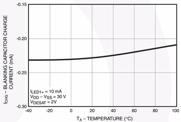
Figure 14. Blanking Capacitor Charge Current ( $I_{CHG}$ ) vs. Temperature
