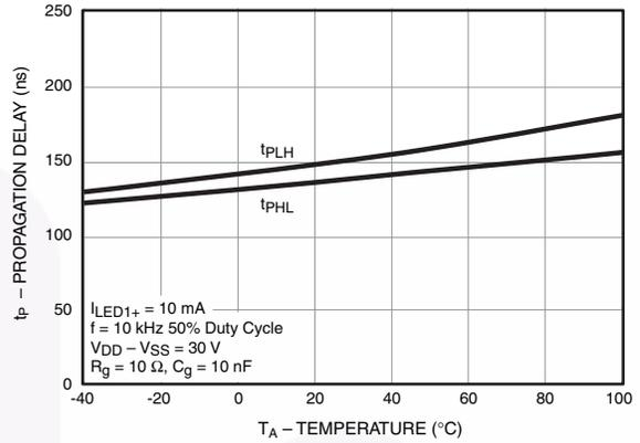
Figure 18. Propagation Delay ( $t_p$ ) vs. Temperature
