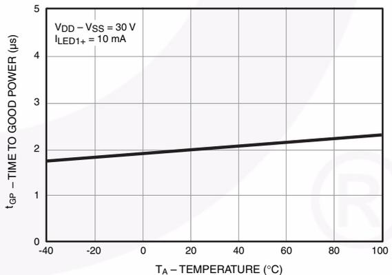
Figure 28. Time to Good Power ( $t_{GP}$ ) vs. Temperature
