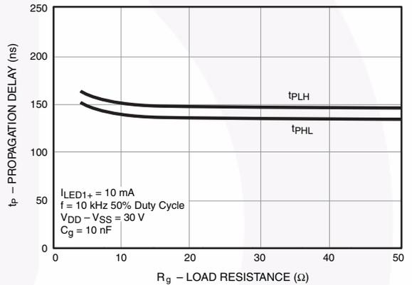
Figure 20. Propagation Delay ( $t_p$ ) vs. Load Resistance ( $R_g$ )
