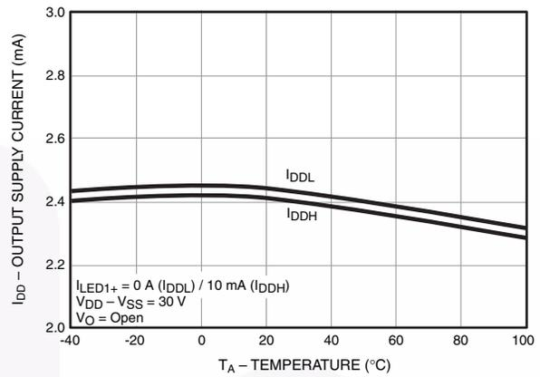
Figure 12. Output Supply Current ( $I_{DD}$ ) vs. Temperature
