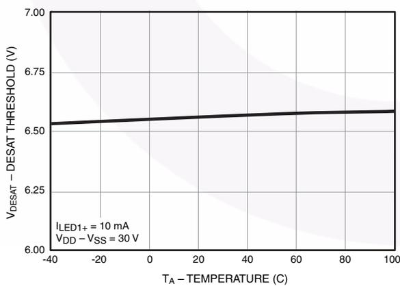
Figure 15. DESAT Threshold ( $V_{DESAT}$ ) vs. Temperature
