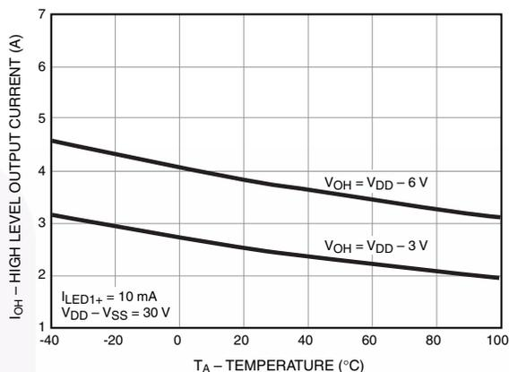
Figure 6. High Level Output Current ( $I_{OH}$ ) vs. Temperature
