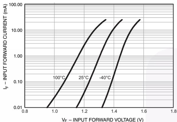
Figure 5. Input Forward Current ( $I_F$ ) vs. Voltage ( $V_F$ )
