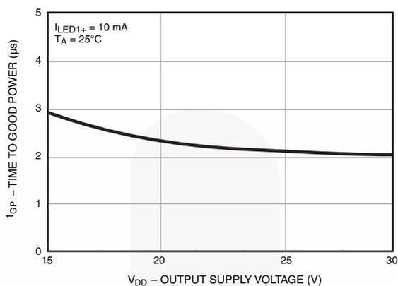
Figure 29. Time to Good Power (t<sub>GP</sub>) vs. Output Supply Voltage (V<sub>DD</sub>)
