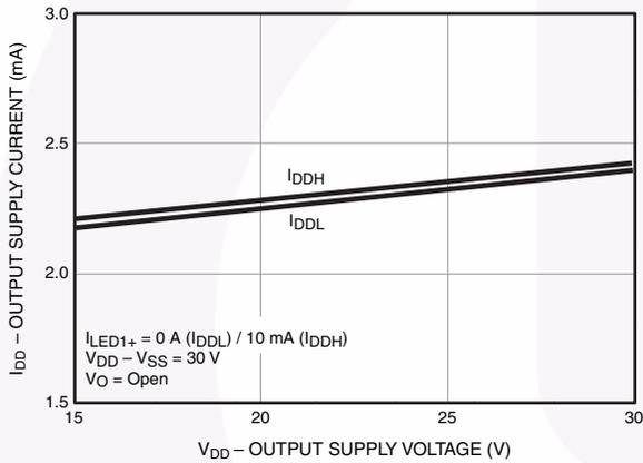
Figure 13. Output Supply Current ( $I_{DD}$ ) vs. Voltage ( $V_{DD}$ )
