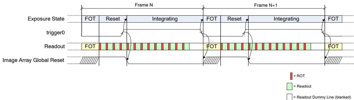
Figure 19. Exposure Time Control in Global-Slave Mode
