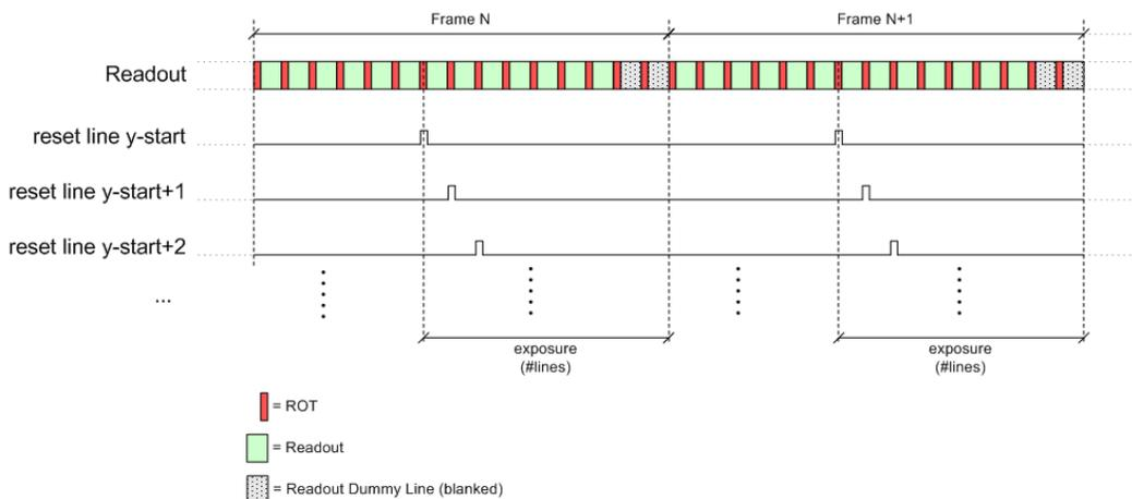
**Figure 20. Integration Control in Rolling Shutter Mode**
