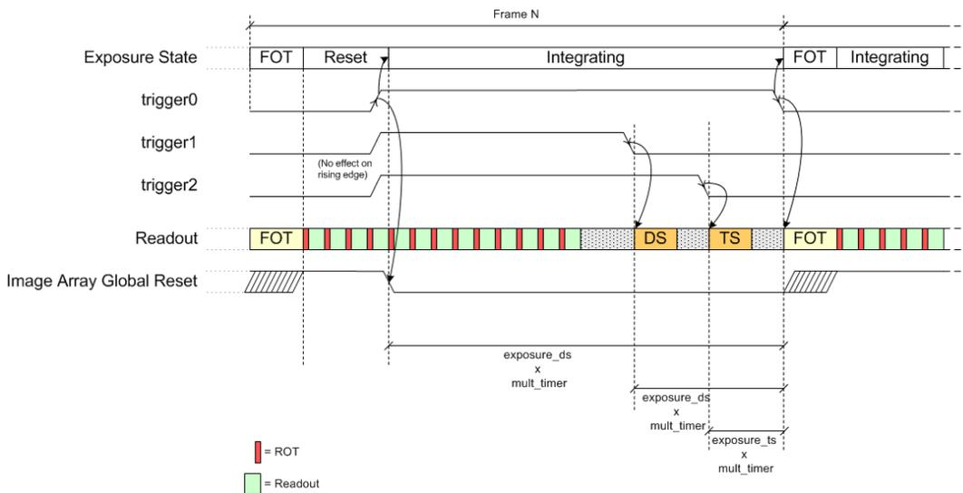
Figure 27. Multiple Slope Operation in Slave Mode
