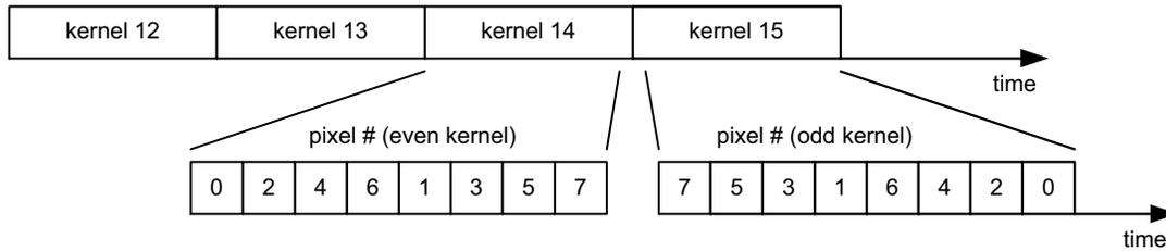
**Figure 39. V2-SN/SE: Data Output Order without Subsampling**
