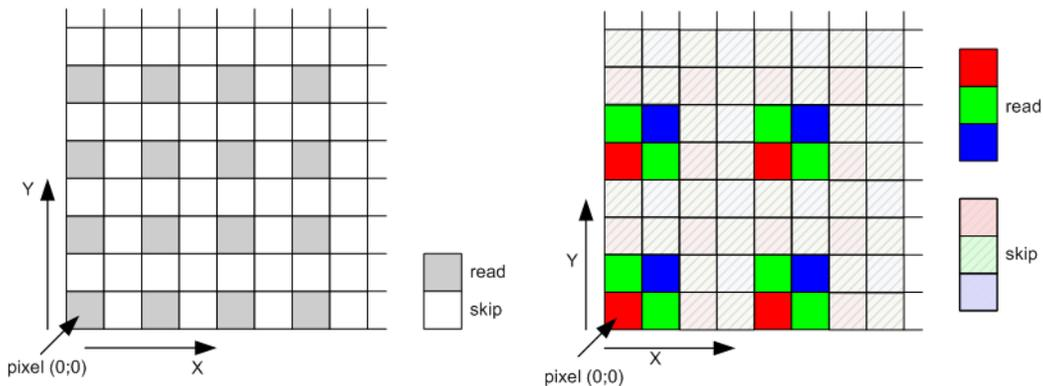
**Figure 24. Subsampling Scheme for Monochrome and Color Sensors**
