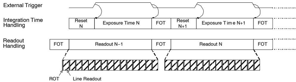
**Figure 8. Pipelined Shutter Operated in Slave Mode**
