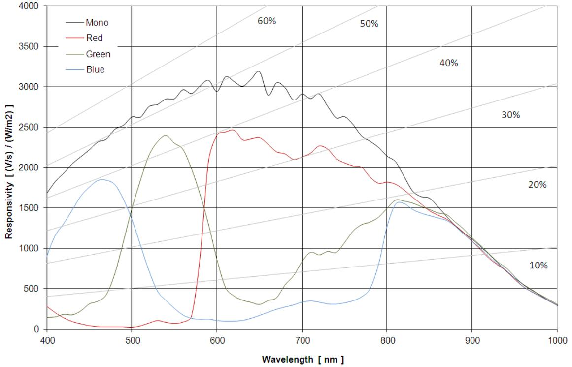
**Figure 3. Spectral Response Curve for Mono and Color**
