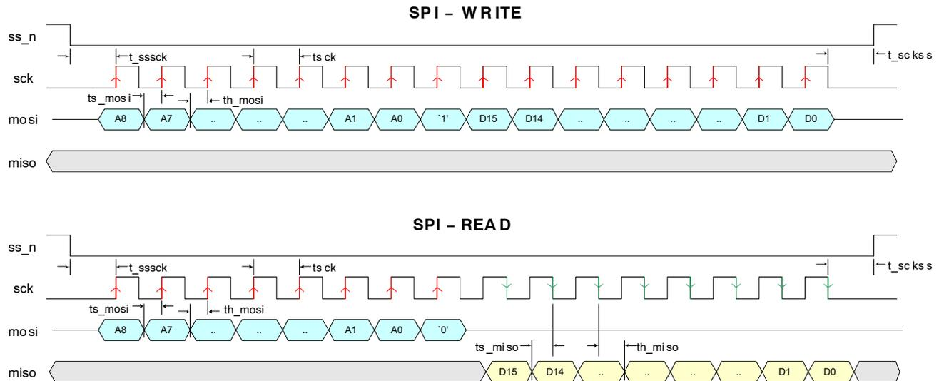
Figure 16. SPI Read and Write Timing Diagram
