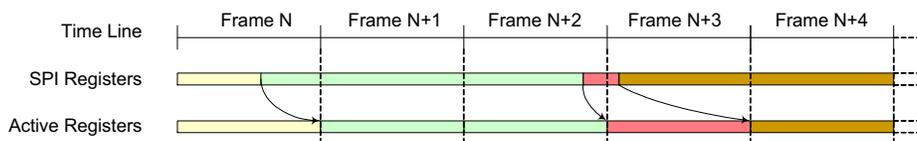
**Figure 14. Frame Synchronization of Configurations (no freezing)**
