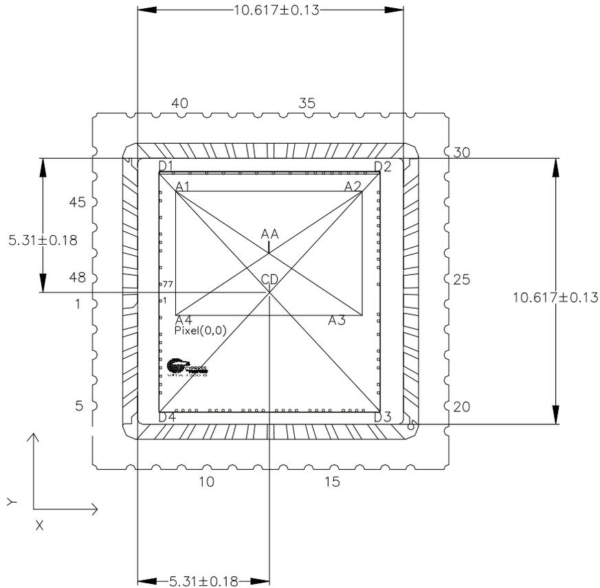
**Figure 43. Graphical Representation of the Optical Center**
