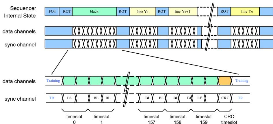
**Figure 30. V1-SN/SE: Time Line for Black Line Readout**
