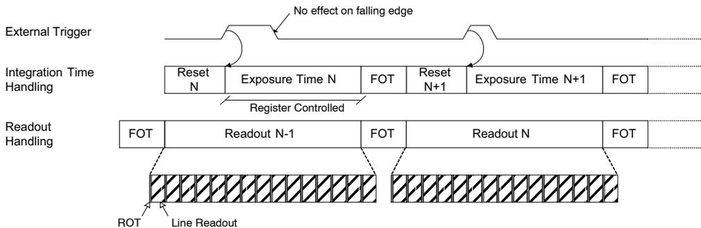
**Figure 9. Triggered Shutter Operated in Master Mode**
