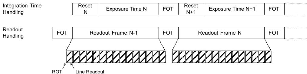
**Figure 7. Integration and Readout for Pipelined Shutter**
