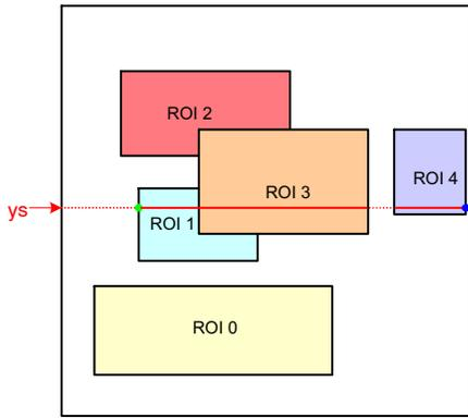
**Figure 23. Scanning the Image Array with Five Windows**
