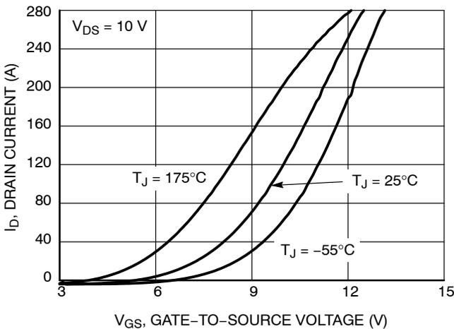
Figure 5. Transfer Characteristics
