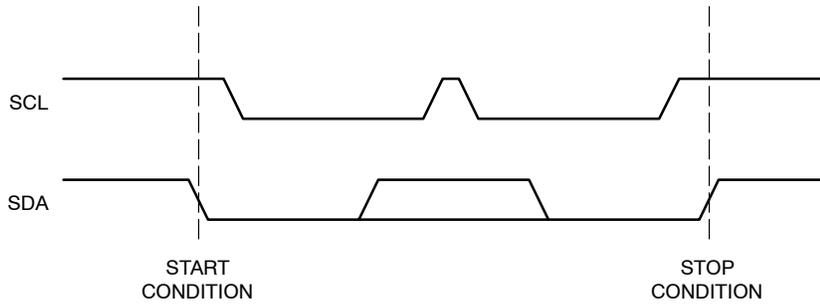
**Figure 2. Start/Stop Timing**
