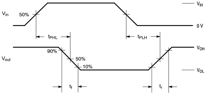
Figure 1. Switching Waveforms
