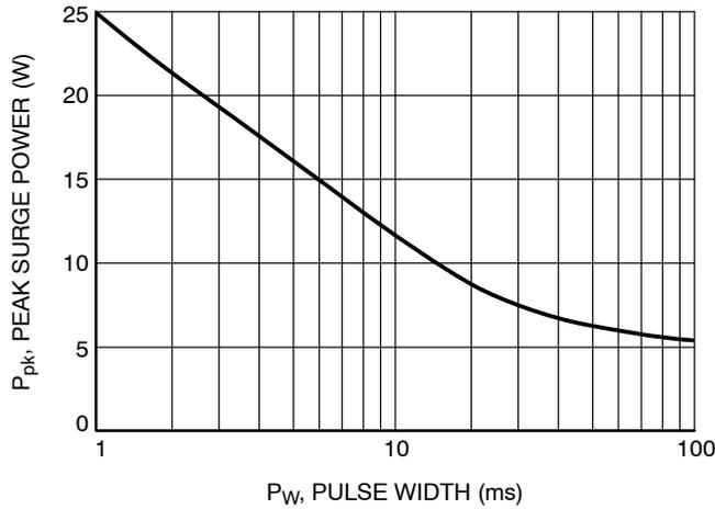
Figure 2. Maximum Non-repetitive Surge Power versus Pulse Width
