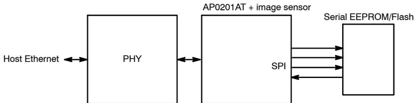
NOTE: In this configuration all settings are communicated to the AP0201AT and sensor through the host.
