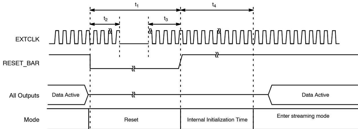
**Figure 6. Hard Reset Operation**
