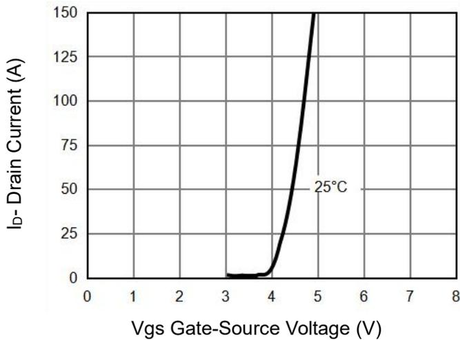
**Figure 2 Transfer Characteristics**
