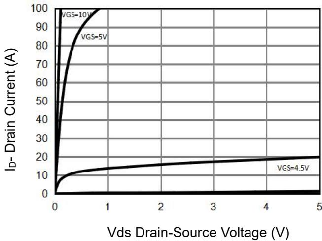
**Figure 1 Output Characteristics**
