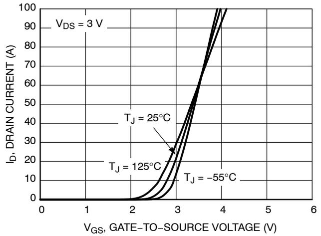
Figure 2. Transfer Characteristics
