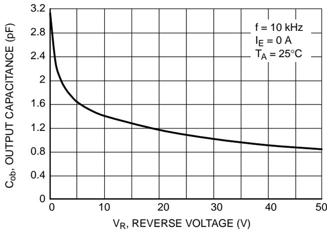
Figure 4. Output Capacitance
