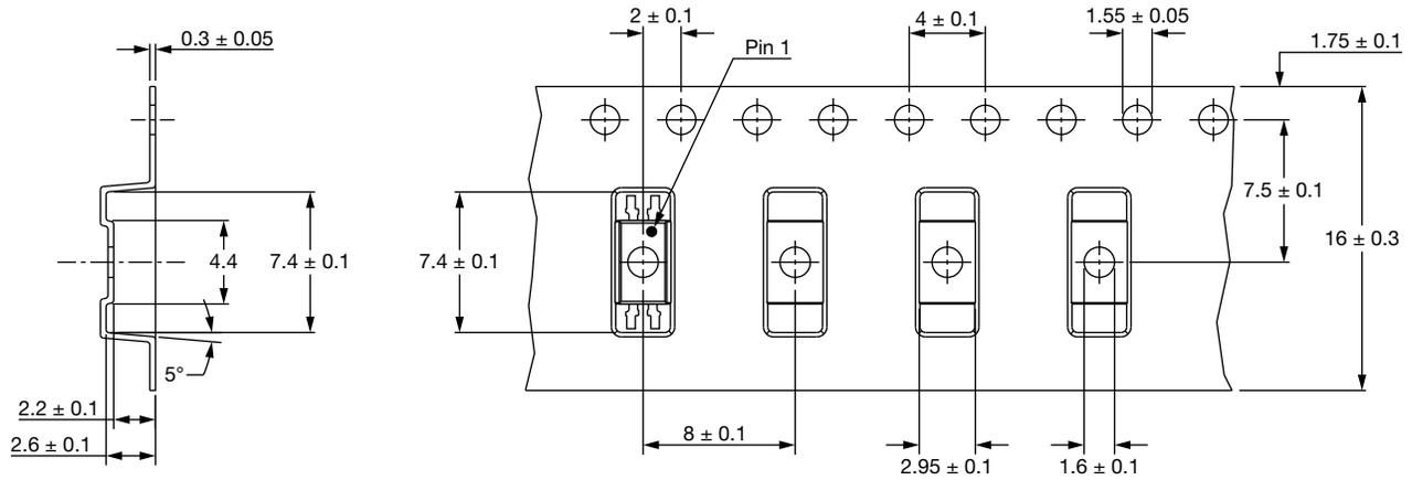
Fig. 18 - Tape and Reel Packing (3000 parts per reel)
