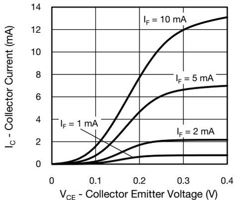
Fig. 8 - Collector Current vs. Collector Emitter Voltage
