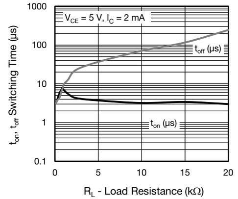
Fig. 16 - Switching Time vs. Load Resistance
