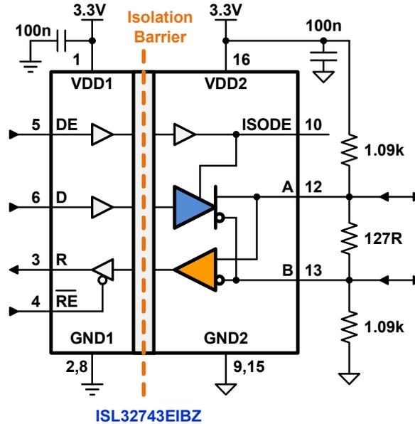
Figure 2. Typical Operating Circuit
