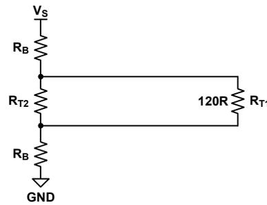
**Figure 8. Failsafe Biasing for a High-speed Data Link**
