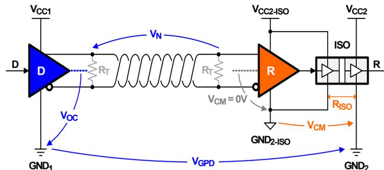
Figure 4. Common-Mode Voltages in an Isolated Data Link
