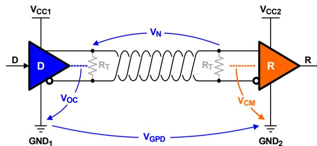
Figure 3. Common-Mode Voltages in a Non-Isolated Data Link
